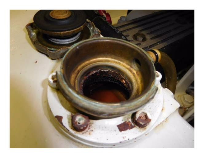
Not to be confused with a recovery tank or bottle, the expansion tank on closed cooling system engines is part of the pressurized cooling circuit; it's typically where the pressure cap is located.
