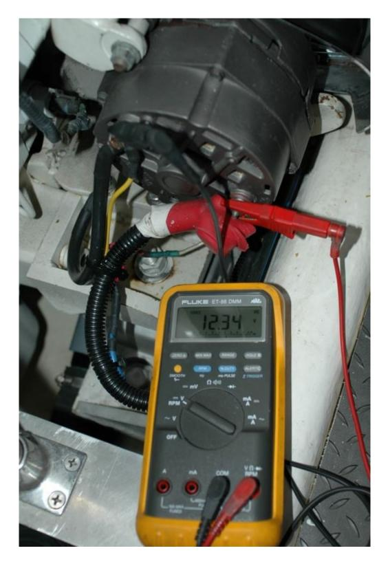
Multimeter voltage measurements are always made in parallel, with the red and black leads connected to positive and negative terminals respectively.
