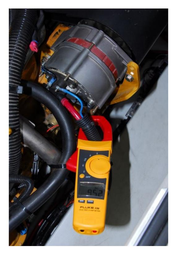
Current or ampere measurements are made in series, with the multimeter becoming part of the circuit. For current measurements above about 10 amps an inductive amp clamp, like the one shown here, is often used.
