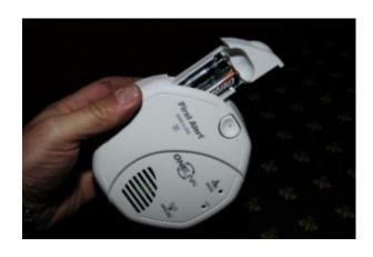
This smoke alarm is capable of communicating with, and setting off other units like it throughout the vessel. The value of this type of alarm cannot be over-estimated. For the cost, it's very likely the cheapest insurance you will ever buy.
