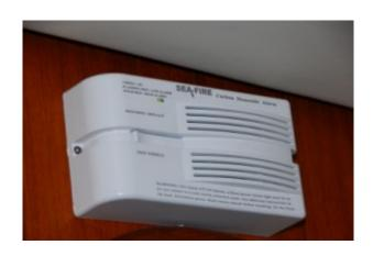
Stand-alone carbon monoxide detectors that are powered from the vessel's own DC system, like the one shown here, are equally as important and necessary as smoke detectors. Internal battery-powered units are just as effective, however, users must remember to replace batteries religiously.
