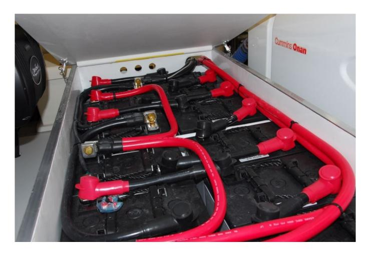
Large battery banks are prone to sulfation because they are frequently chronically undercharged.
