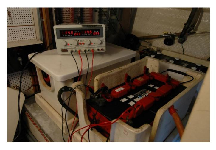
A controlled over-charge, known as equalization or conditioning, is carried out using either an adjustable current/voltage bench charger, shown here, or a vessel's own charger that has an equalization function.
