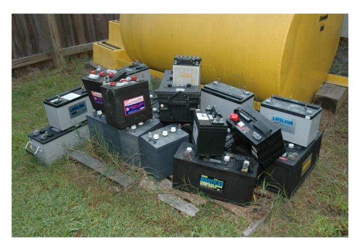
Many batteries die an unnecessary, premature death, the victims of undercharging and sulfation.
