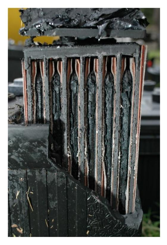
Sulfation occurs when battery plates are corrupted by inert crystals, every one of which displaces active material, thereby diminishing a battery's capacity.
