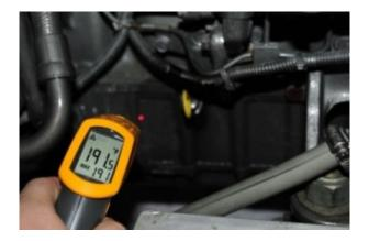
The infrared pyrometer, when used properly, can provide a wealth of information. In this case it's confirming that the oil temperature is correct while under load. As useful as they are, pyrometers can be, and often are, used incorrectly.
