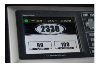
A clean bill of health, this electronically controlled engine offers a wealth of valuable information in its display, and the news here is all good. The engines reaches its WOT (and just a little more, which is desirable) at 100% throttle and 99% load. Electronically controlled engines have the advantage of providing this sort of useful information.
