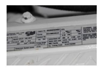
Most engines include a commission tag or plate that details, among other things, the engine's maximum rated rpm.
