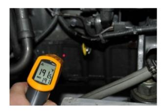
The infrared pyrometer, when used properly, can provide a wealth of information. In this case it's confirming that the oil temperature is correct while under load. As useful as they are, pyrometers can be, and often are, used incorrectly.
