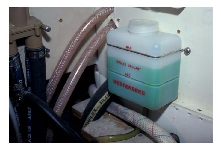
Coolant recovery bottles are available in a range of shapes and sizes. Bottle selection is driven by the overall volume of the cooling system, larger systems require larger bottles.
