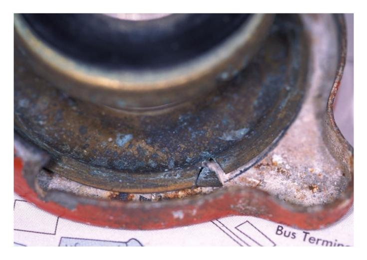
Not all cooling system pressure caps are alike. Those with a brass upper bushing are not designed to be used with recovery bottles; and the bushings, like the one shown here, are prone to cracking.
