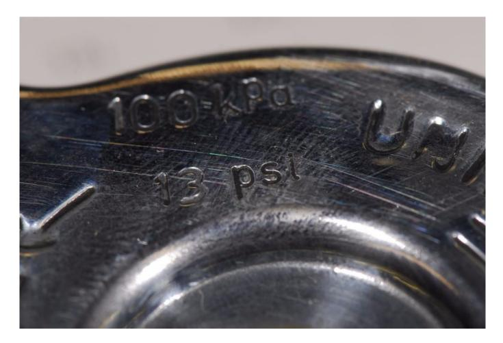
Pressure caps carry pressure ratings, which are nearly always embossed on their surface. Using a cap that carries the proper pressure rating is critically important; if it's too high it can lead to leaks, if it's too low it may not provide proper boil and cavitation protection.
