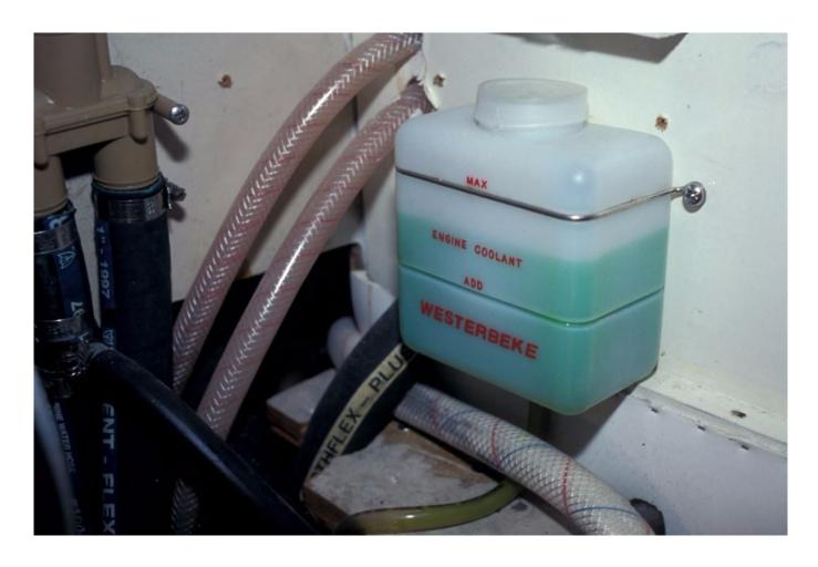
Coolant recovery bottles are available in a range of shapes and sizes. Bottle selection is driven by the overall volume of the cooling system, larger systems require larger bottles.
