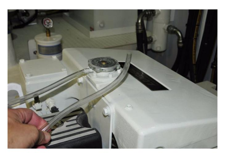
While it's all too commonly used, clear PVC hose is not robust enough for coolant applications, it collapses, chafes and melts far too easily. Type B fuel hose makes for a far better choice.
