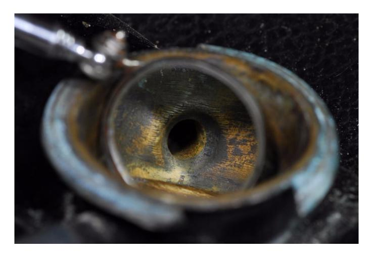
The port located in the expansion tank fill neck allows coolant to flow to the recovery bottle when the cap reaches
