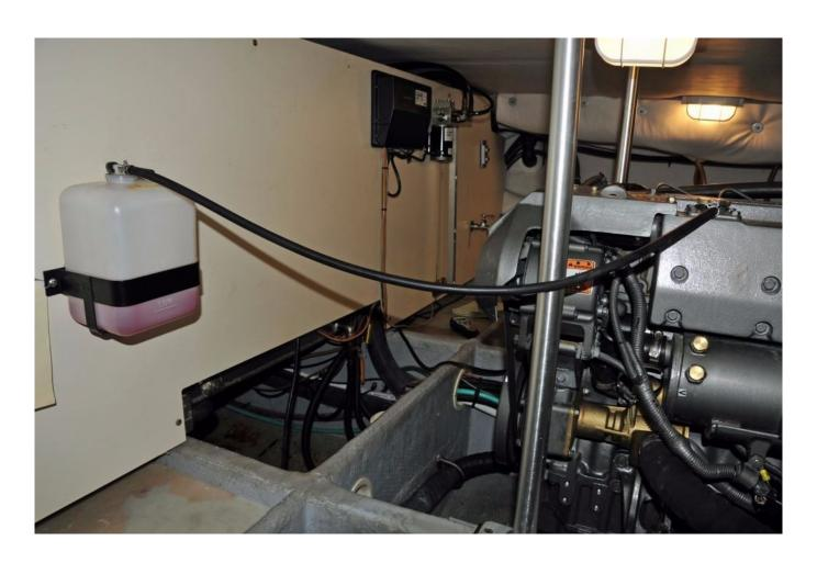
Coolant recovery bottle plumbing should be routed so that it is not in harm's way, and so that it does not impede access around the engine. Most recovery bottles are plumbed from the bottom, however, some, like the one shown here use an internal pick up tube.
