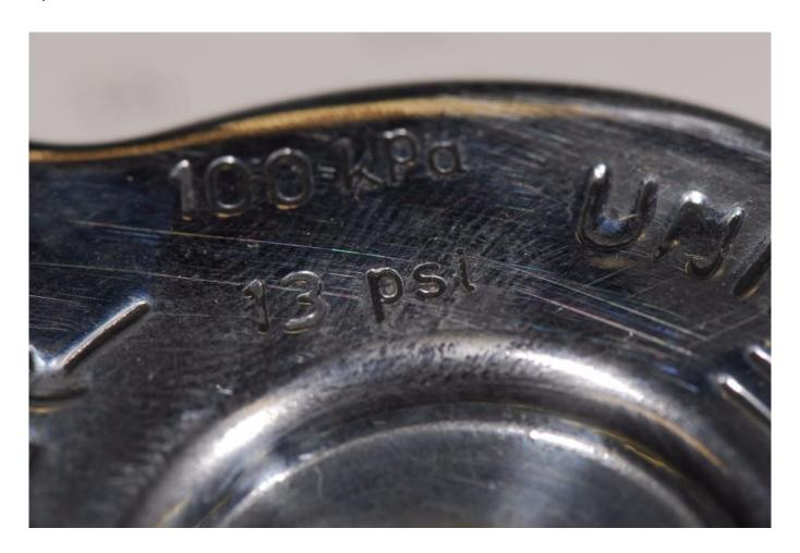
Pressure caps carry pressure ratings, which are nearly always embossed on their surface. Using a cap that carries the proper pressure rating is critically important; if it's too high it can lead to leaks, if it's too low it may not provide proper boil and cavitation protection.
