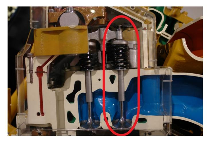
A cut-away view of a cylinder head, showing a complete valve assembly (this engine uses dual intake valves). Fresh air would travel through the intake manifold, painted blue here, and then proceed down into the cylinder or combustion chamber.
