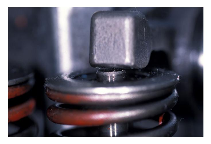
The interface between rocker arm and valve stem; a small gap can be seen in this image. It is between these two components where valve clearance is measured.
