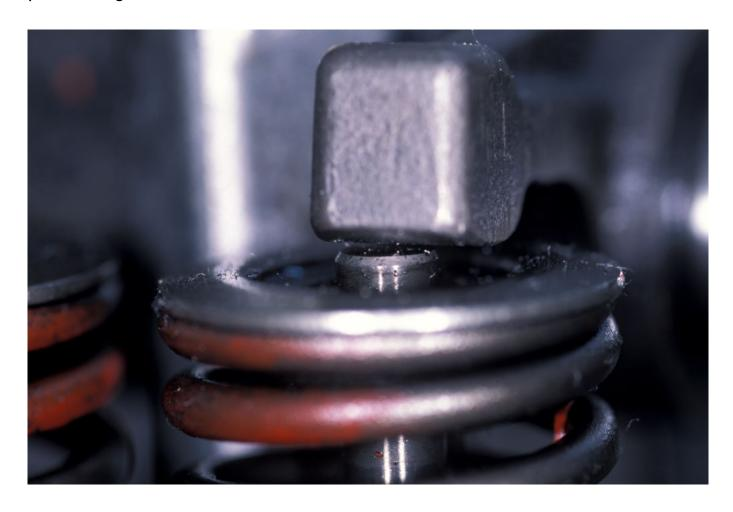
The interface between rocker arm and valve stem; a small gap can be seen in this image. It is between these two components where valve clearance is measured.
