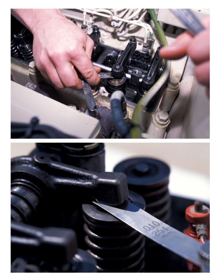
Here, valve clearance is being checked using a conventional feeler gauge.
