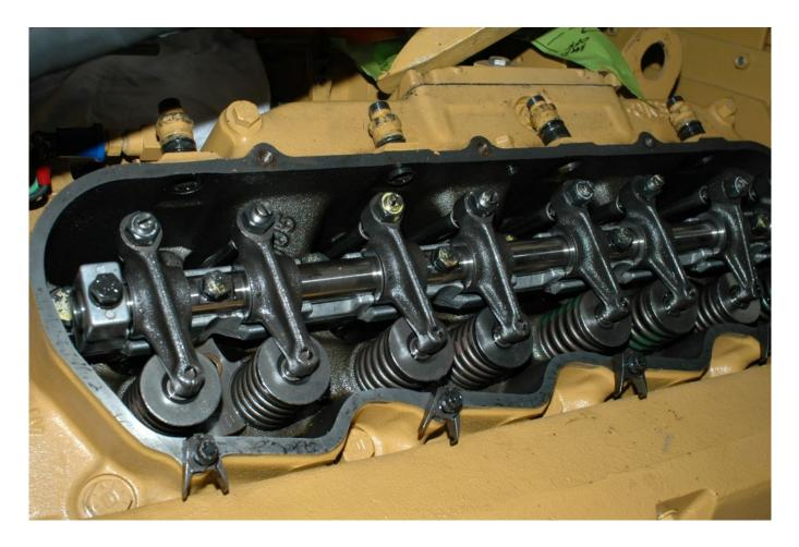
Rocker arms, rocker arm shaft, and valve springs can all be seen in this image, the valves themselves reside within the spring and under the head and are thus not visible.
