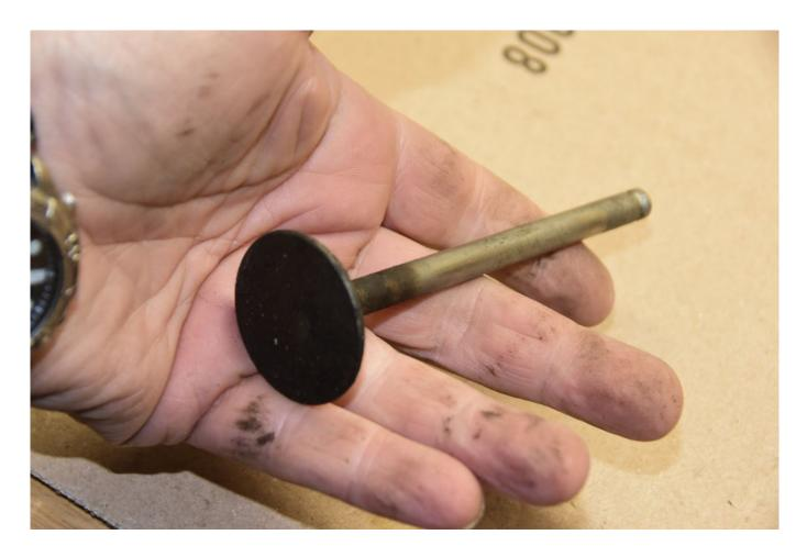
While they are moving parts, intake and exhaust valves themselves are simple components. Here the author holds an intake valve (from his vintage Triumph roadster).
