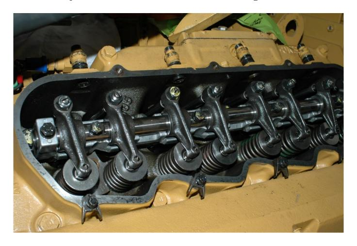
Rocker arms, rocker arm shaft, and valve springs can all be seen in this image, the valves themselves reside within the spring and under the head and are thus not visible.
