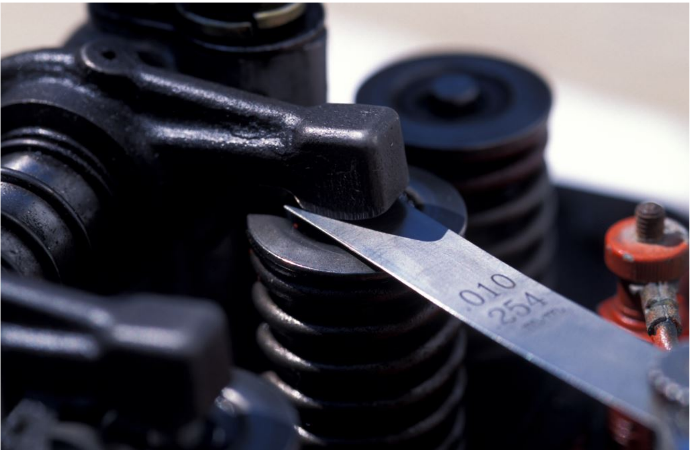
Here, valve clearance is being checked using a conventional feeler gauge.
