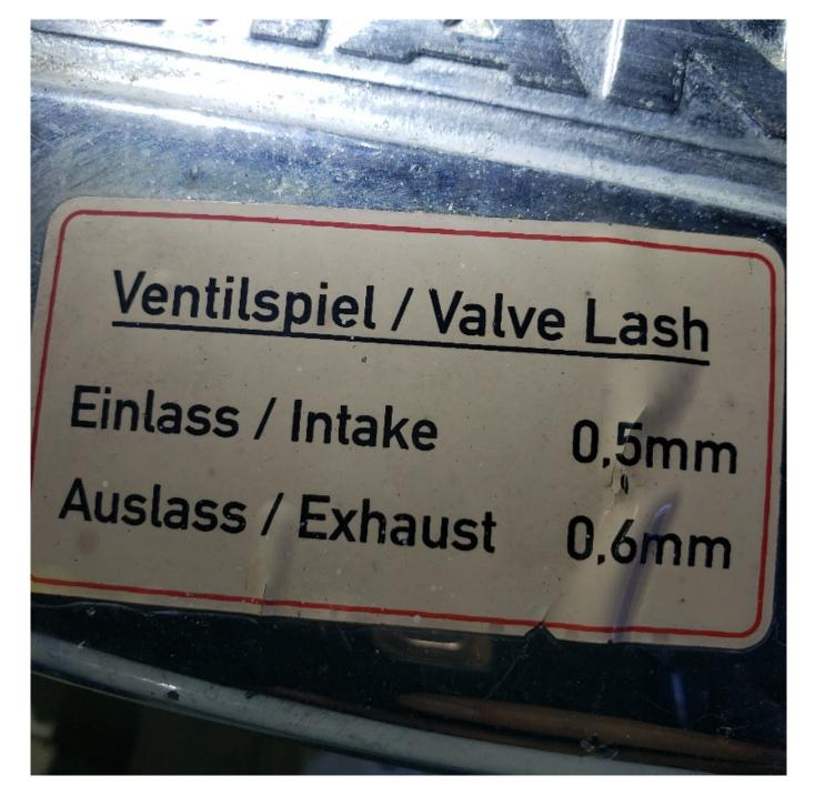
Valve clearances are provided by engine manufacturers, in this case on a decal posted on the valve cover so it can't be missed.
