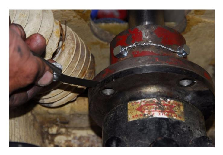
Tried and true, using feeler gauges to measure and close the gap between propeller shaft and transmission output couplings.
