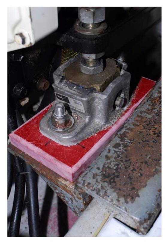
Motor mounts carry out a Herculean task, supporting the engine and absorbing both vibration and thrust, however, they are the primary means of adjustment for alignment. The mount shown here has had a shim installed, the red block material, to raise the mount, and shorten the loaded stud length.
