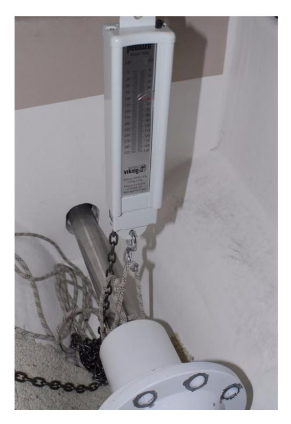
Eliminating shaft droop can be accomplished using a hanging or conventional scale, thereby accounting for the weight of the shaft and coupling.
