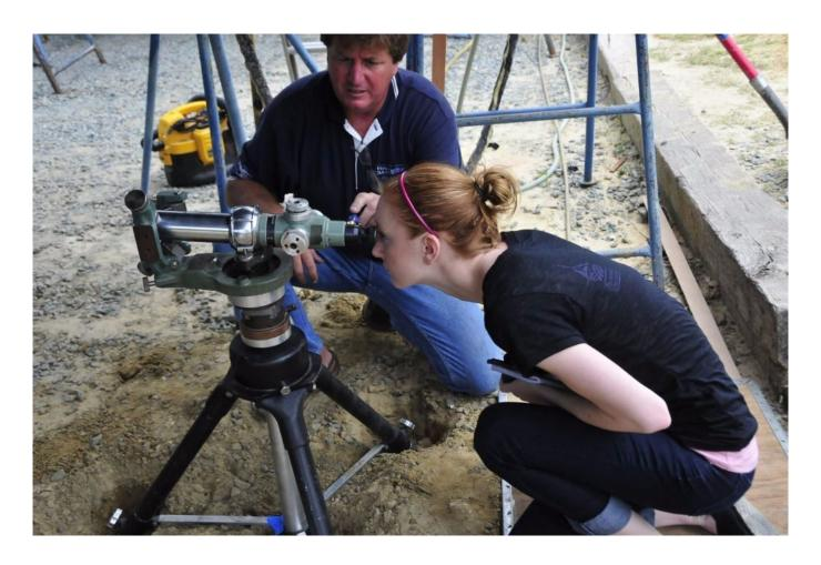
Optically "sighting through" to, among other things, avoid aligning the transmission output coupling to a sagging or drooping shaft, is a critical aspect of the alignment process.
