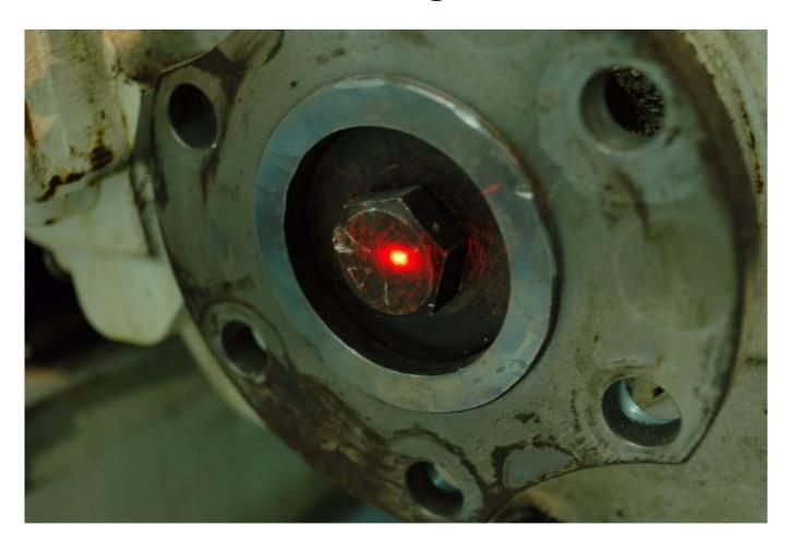
A laser can be used to "sight through" a shaft. Here the
