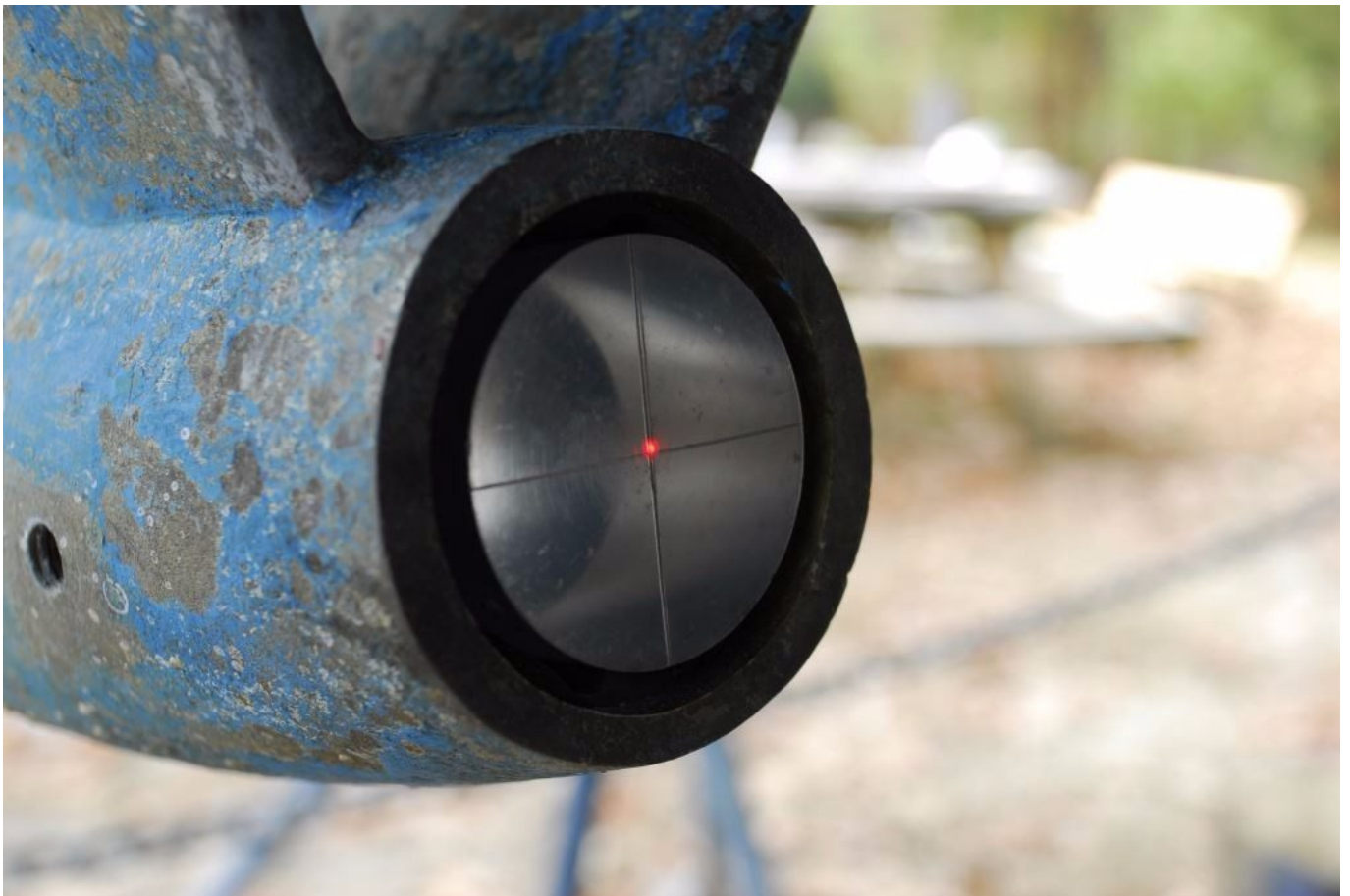
Bearing alignment can be analyzed using either optical (top)
