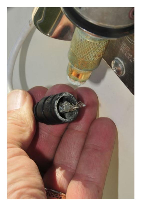
This coaxial cable easily separated from its terminal, likely because it was not properly installed. The boot shown here, while seemingly desirable, can actually retain water. Heat shrink tubing or electrical tape is preferred.
