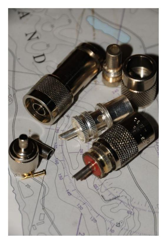
A selection of coaxial terminals, each specifically designed for a particular cable type.
