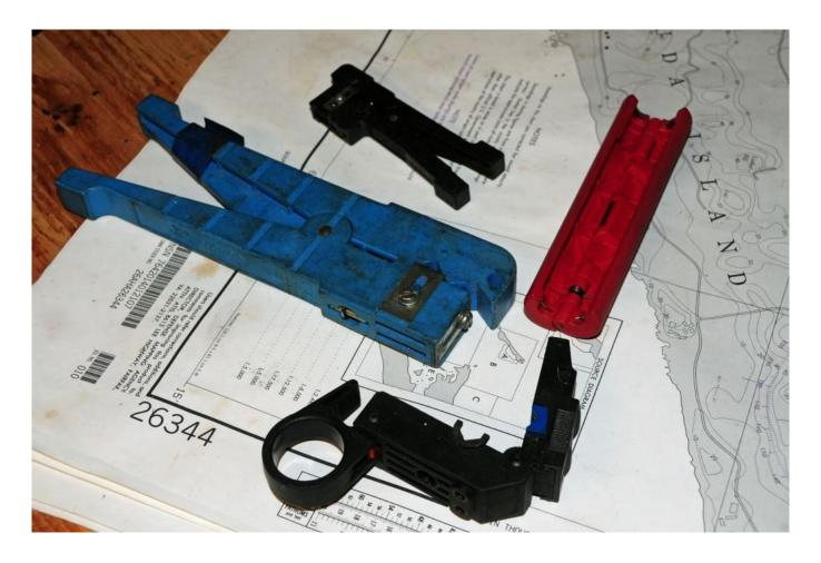
While it can be done manually, those preparing coaxial cable for terminal installation should utilize readily available special tools.
