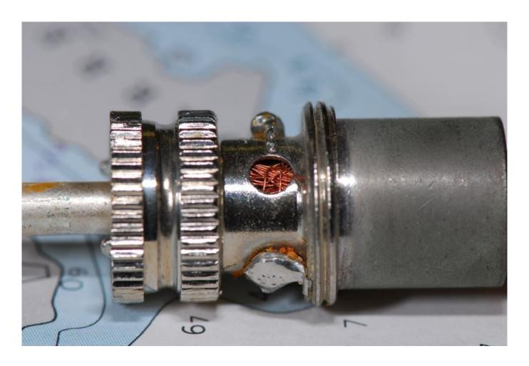
Properly soldering coaxial terminals requires practice. These "cold" solder joints are unacceptable, and all holes should be filled.
