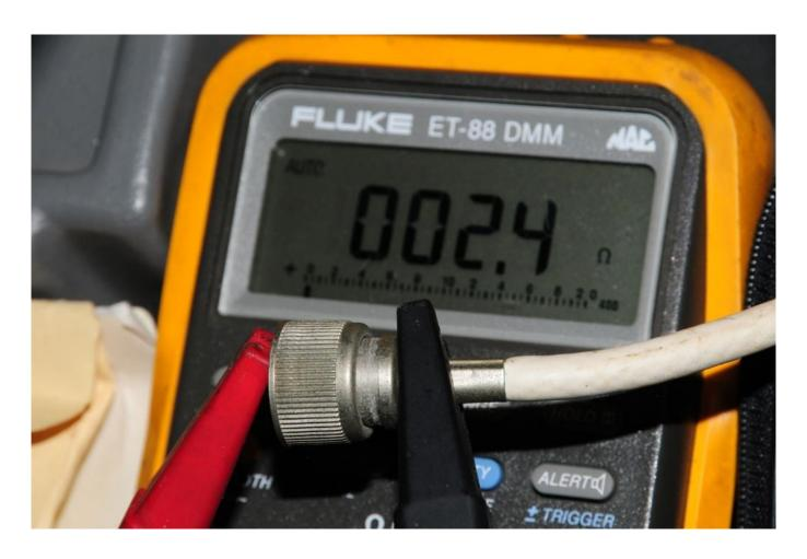
Testing cables using an ohm meter, after terminals are installed, can identify shorts and open circuits before the installation is complete.
