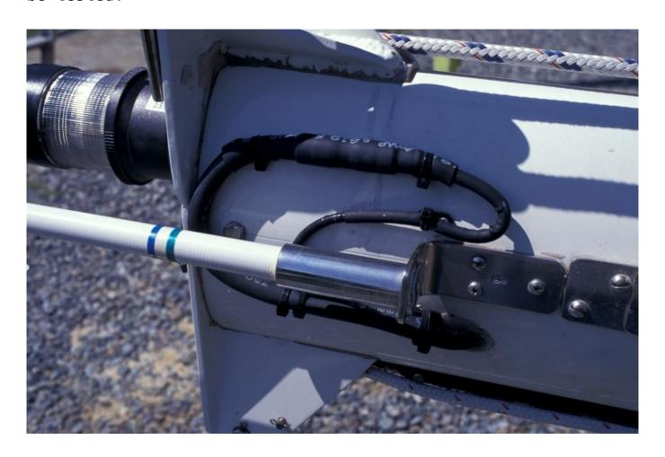
A heavy low loss cable transitions to a smaller diameter "pigtail" cable, one that's permanently attached to the antenna. While the bend in the smaller cable is too sharp, the heat shrink tube waterproofing is ideal.
