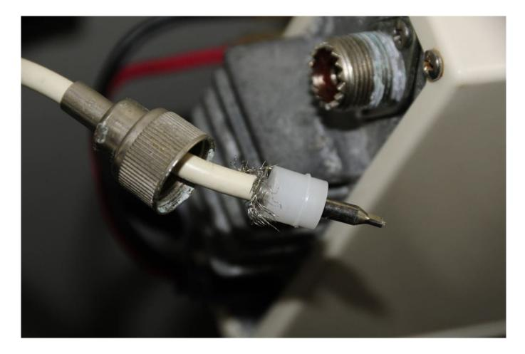
Great care must be taken when installing coaxial terminals. A single errant shield strand, making contact with the center conductor, will cause a short and diminish performance.
