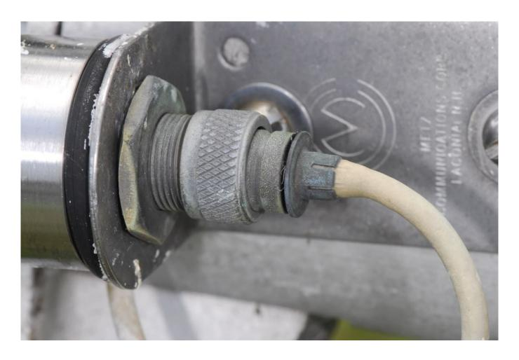
A poorly made connection, it lacks water proofing. Note the visible shield strands, these will act as wicks for water entry into the cable.
