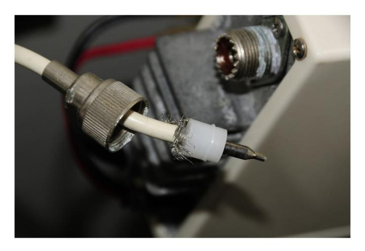
Great care must be taken when installing coaxial terminals. A single errant shield strand, making contact with the center conductor, will cause a short and diminish performance.
