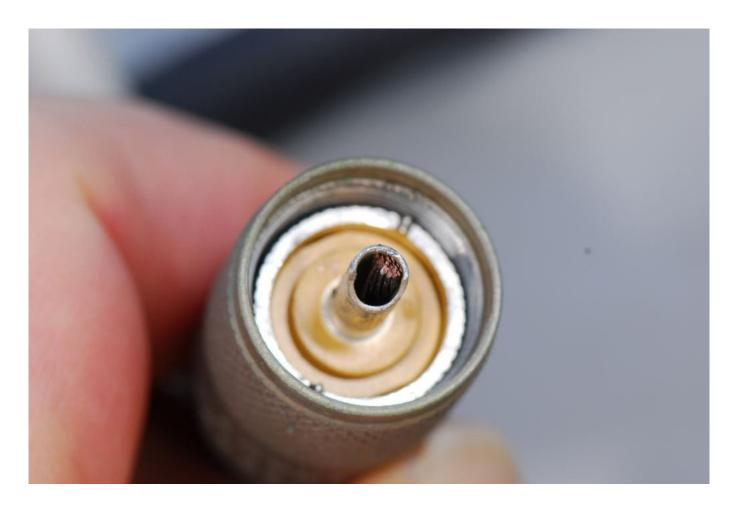
Failing to use solder on coaxial terminals that are designed
