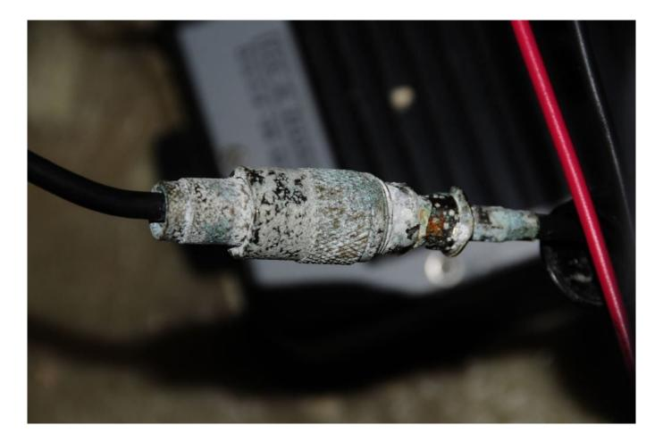
Exposed coaxial terminals will corrode. In wet locations, including bilges, they should be installed using a light film of dielectric grease, and then covered with heat shrink tubing or high quality electrical tape; if on weather decks these must be UV resistant.
