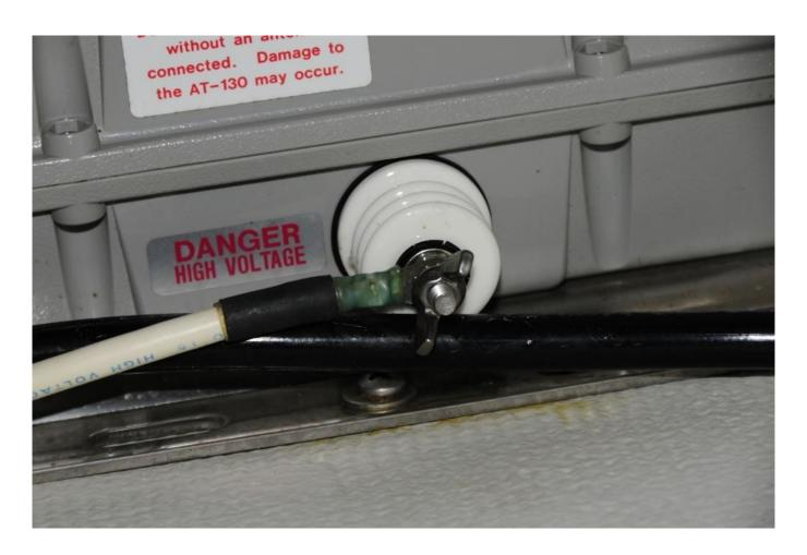
The connection between an SSB tuner and the antenna relies on GTO cable, which is vastly different than coaxial cable. It acts as part of the antenna, and the terminal on the tuner, shown here, should be insulated.
