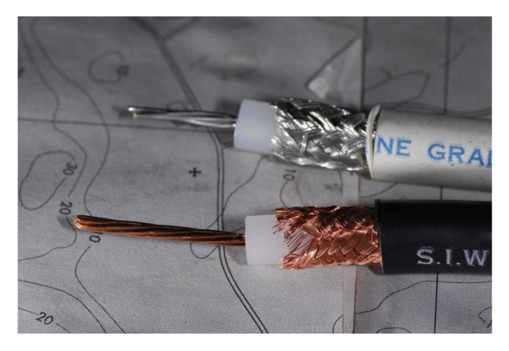
While tinned, corrosion resistant conductors are desirable, some very low loss cable is not available in this format. Given the choice, choose low loss over corrosion resistance. Careful attention should be paid to waterproofing installations regardless of the type of cable that is used.
