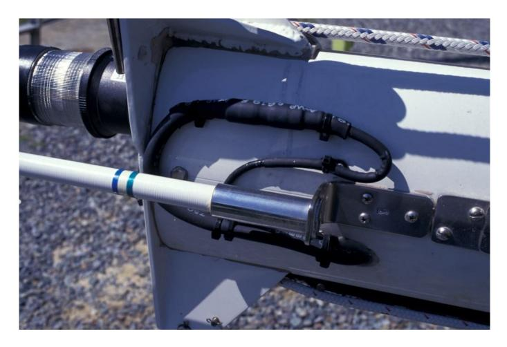
A heavy low loss cable transitions to a smaller diameter "pigtail" cable, one that's permanently attached to the antenna. While the bend in the smaller cable is too sharp, the heat shrink tube waterproofing is ideal.
