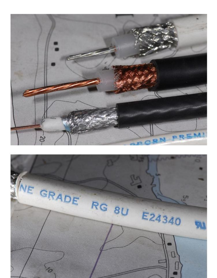
Coaxial cable is available in a range of sizes, types, and
