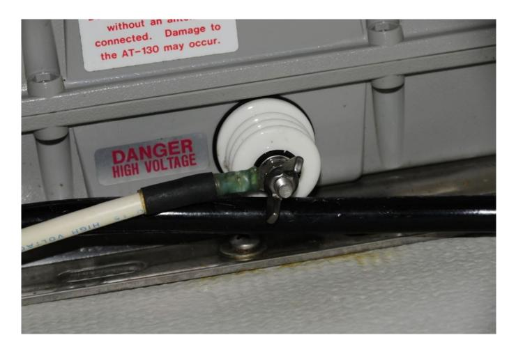
The connection between an SSB tuner and the antenna relies on GTO cable, which is vastly different than coaxial cable. It acts as part of the antenna, and the terminal on the tuner, shown here, should be insulated.
