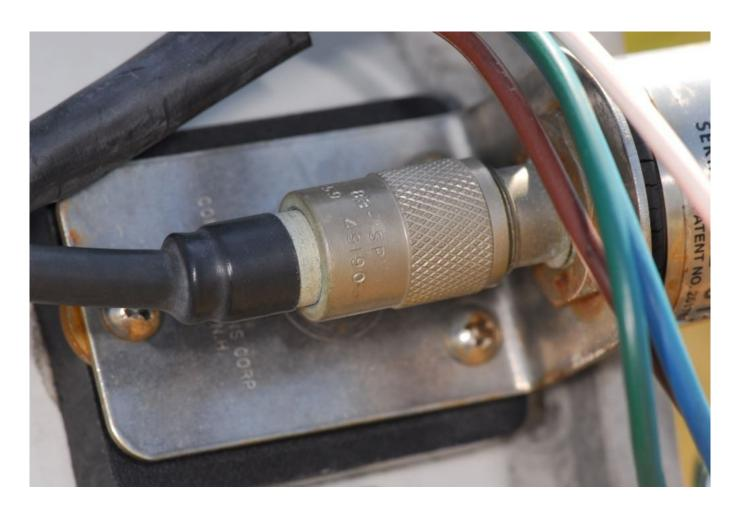
Ideally, this terminal should be completely enclosed in heat shrink tubing.
