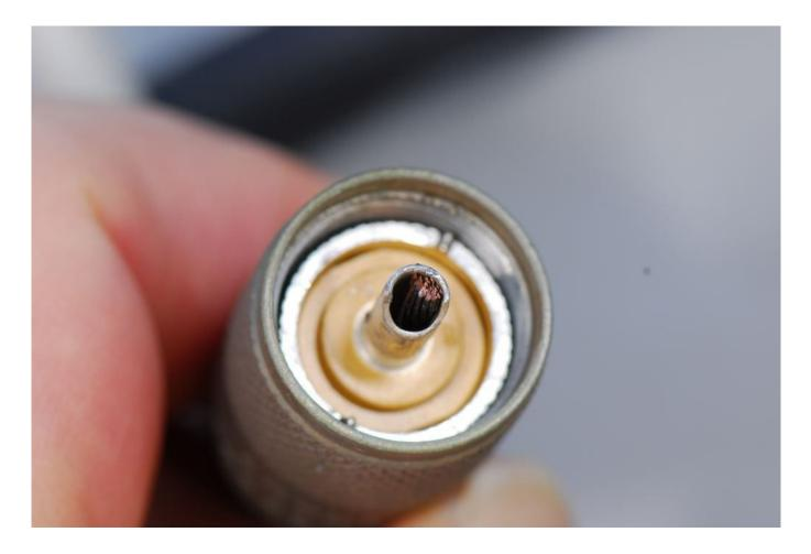
Failing to use solder on coaxial terminals that are designed
