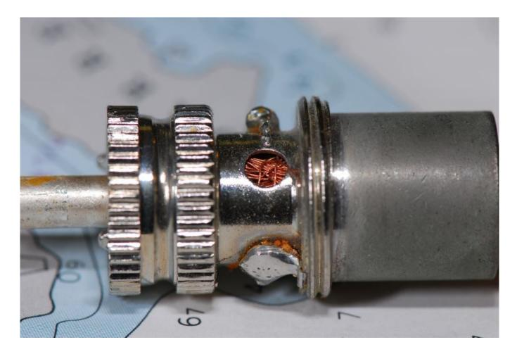
Properly soldering coaxial terminals requires practice. These "cold" solder joints are unacceptable, and all holes should be filled.
