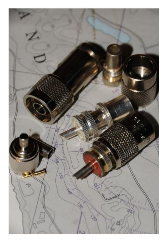
A selection of coaxial terminals, each specifically designed for a particular cable type.
