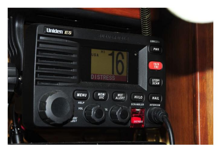
For VHF installations, the only way to be certain the system is performing properly is to obtain a radio check form a distant station, one that is no less than 10 nm. away.
