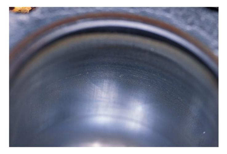
The cross hatch, essential oil-retaining grooves cut into cylinder walls, has been completely worn off the walls of this generator's cylinder walls (above), the result of chronic low load operation. Compare this with "healthy" cross hatch pattern (top).
