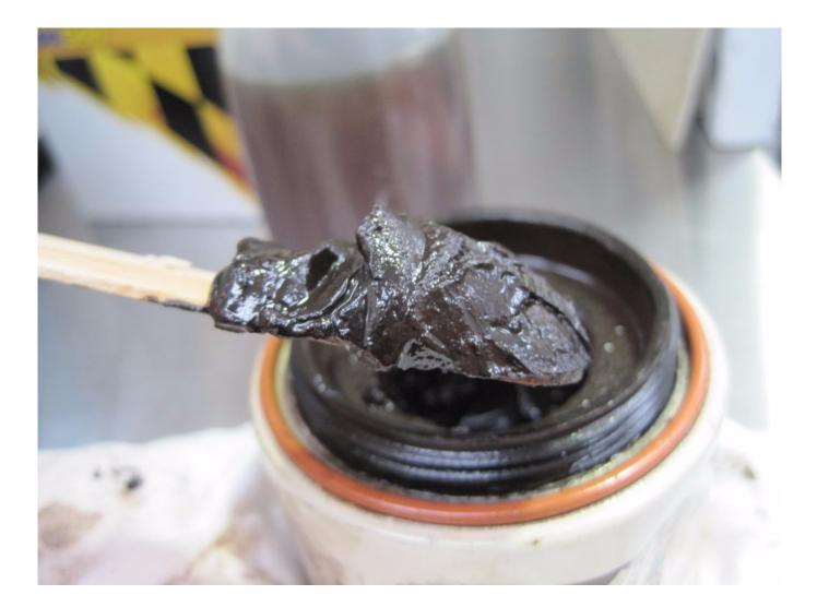
Chronic low load operation often leads to sludge formation, an extreme case is shown here, within crankcases, which can impair lubrication of valve trains, timing chains and other components.
