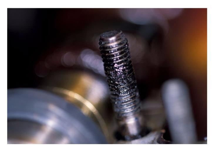
After sludge comes varnish, the latter is far more damaging in that it is hard and plastic-like, similar to varnish, and can easily clog oil galleries and ports.
