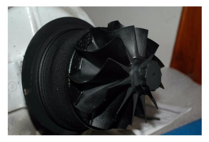
Yet another undesirable side effect to under loading, "wet stacking" a process where un-burned fuel and soot accumulate in turbo chargers and exhaust systems, thereby impairing their efficiency.
