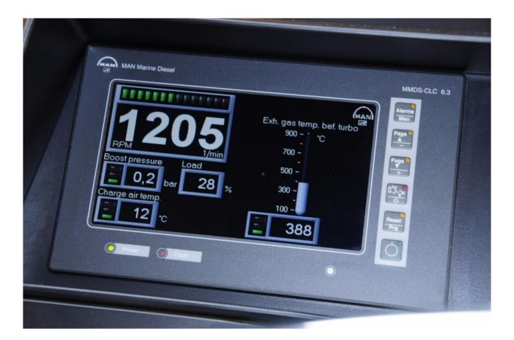
Oil and exhaust temperature tell the real story where the under loading phenomenon is concerned. Few engine instruments show oil and exhaust gas temperature, this one is an exception, showing 95°C, or 203°F for oil, and 400°C or 750°F for exhaust, both of which are ideal.
