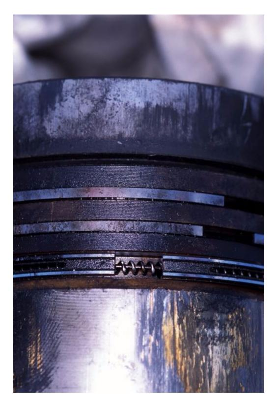
Under loading can lead to piston ring soot clogging, which in turn exacerbates blow-by and oil contamination.
