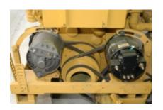
Twin alternators operating on a single engine. When dual alternators are installed in this manner it's preferable to locate them opposite one another in order to balance the load on the crankshaft.
