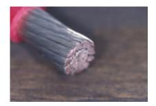
Many fine strands, tinned in this case, make high quality large diameter cable flexible and failure resistant.
