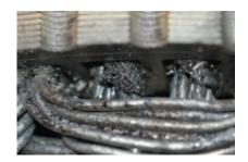
A close up of the overheated windings, note the insulating material has vaporized.
