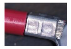
Wire and crimp terminals are the means by which charge current travels to battery banks, and how current travels from the battery bank to house loads. It's imperative that wiring be secure, reliable and installed in a manner that presents the lowest resistance possible.
