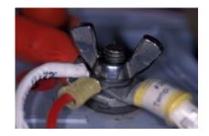
Wing nuts are simply inappropriate for securing battery terminals in any application, especially in high output charging scenarios.
