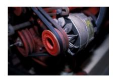
Stock alternators, even ones that appear to have high output, are rarely up to the task of charging large house battery banks.
