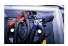
Keep the number of connections at the battery to a minimum, just one or two to a post (four is the absolute limit). Instead, use bus bars that complete connections off of the battery.
