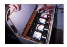
The size of the battery bank is based on the vessel's house needs as well as its ability to be charged.
