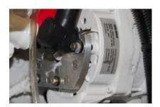
Purpose made high output alternators are designed to produce nearly their full output for extended periods. They can do so by being able to dissipate heat effectively, in some cases by using diodes mounted in external heat sinks.
