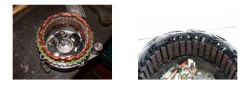
A new alternator (left) and a stock alternator that was externally regulated (right), albeit for a short time. The windings on the alternator on the right have been discolored as a result of overheating (they previously looked like those on the left.
