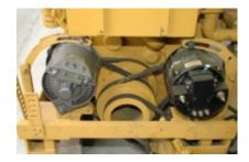
Twin alternators operating on a single engine. When dual alternators are installed in this manner it's preferable to locate them opposite one another in order to balance the load on the crankshaft.
