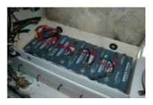
Battery banks must be wired in such a way as to draw current evenly across the bank, rather than from a single end.
