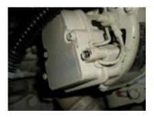
Stock, internally regulated alternators like this one fail miserably when called upon to control charge on house battery banks.
