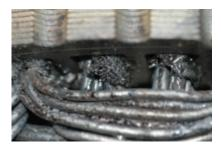
A close up of the overheated windings, note the insulating material has vaporized.
