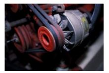
Stock alternators, even ones that appear to have high output, are rarely up to the task of charging large house battery banks.
