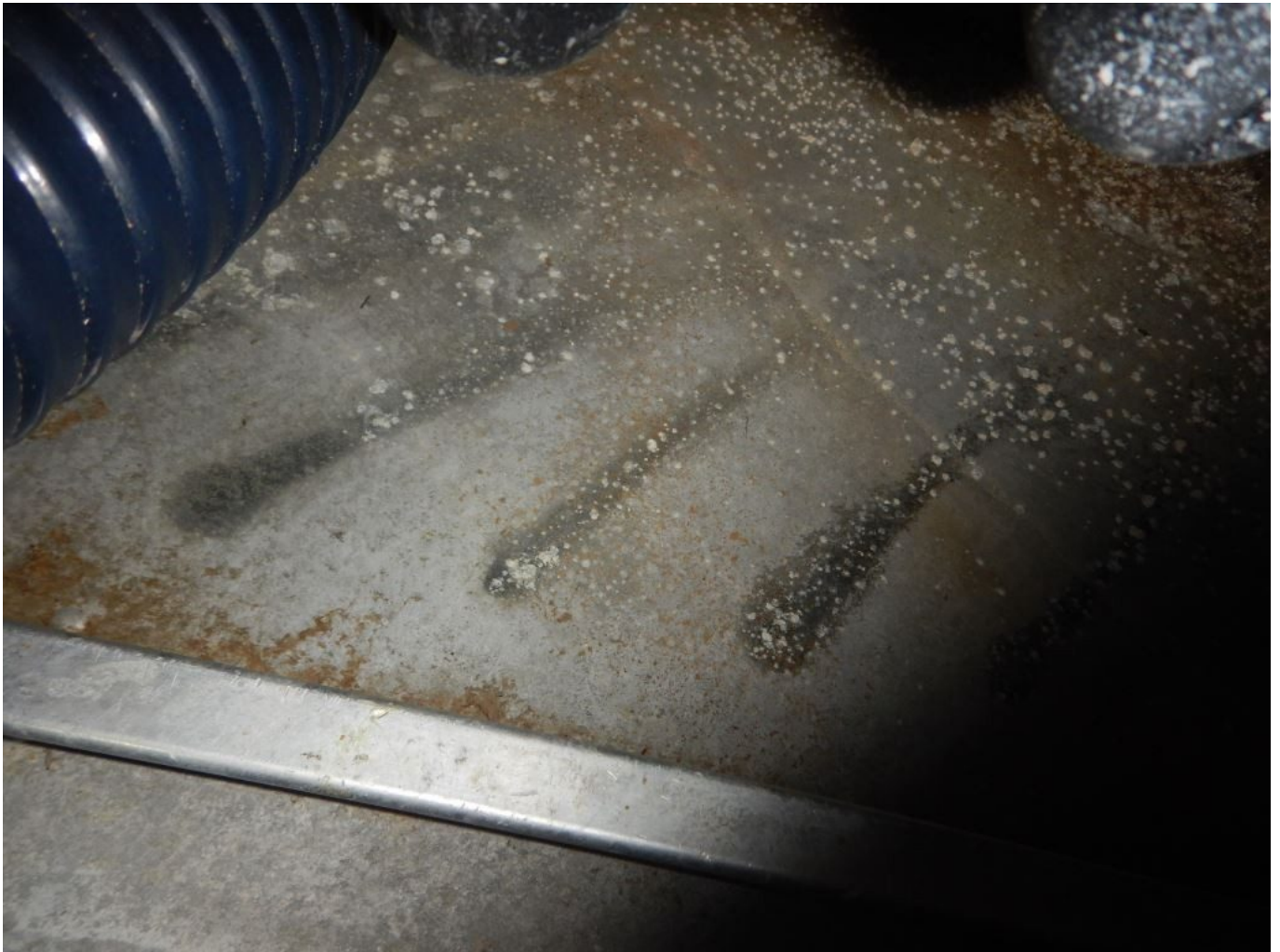
Aluminum hull corrosion, the result of water dripping from a bronze raw water plumbing manifold.
