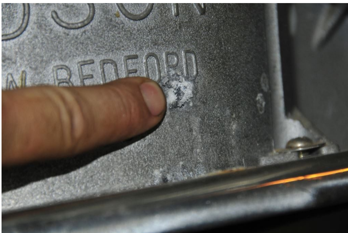
An aluminum body manual bilge pump. Stagnant water trapped
