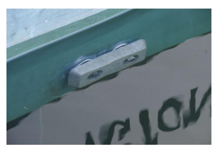
Hull-mounted anodes, these may be zinc, aluminum or magnesium, can be connected to the bonding system, and thereby provide protection for all connected underwater metals.
