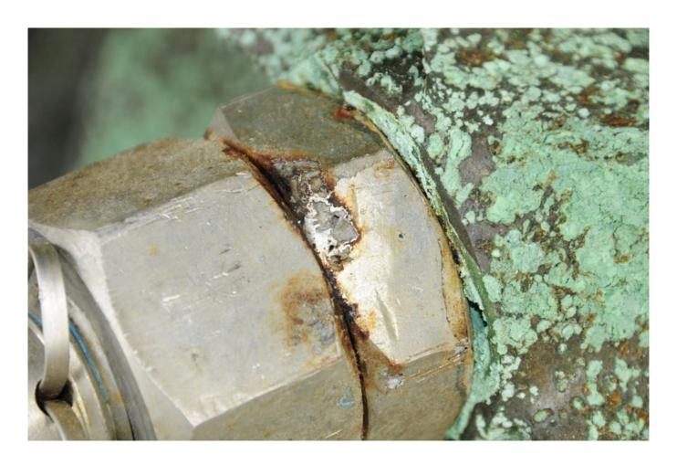
Stray current corrosion is extremely destructive and it occurs comparatively quickly, it qualifies as a corrosion emergency, as it's capable of impacting a vessel's watertight integrity in a matter of days if not hours.
