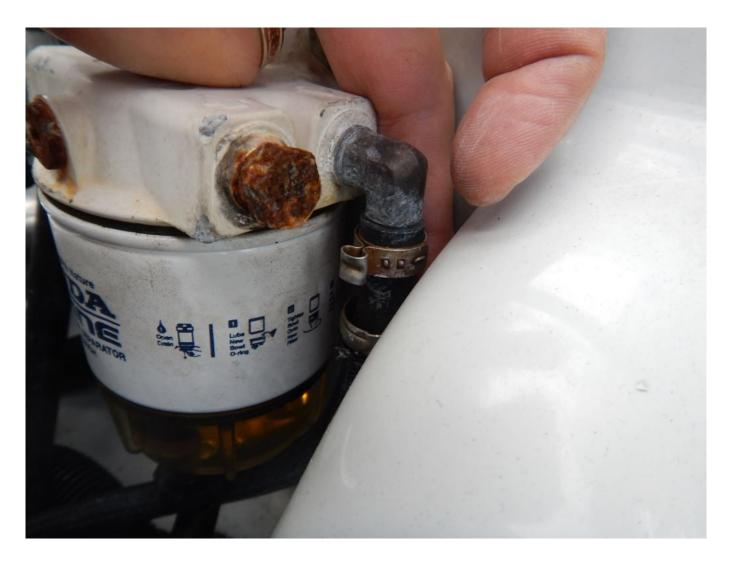
Aluminum fuel filter housings like the one shown here are often plumbed with galvanically incompatible brass pipe to
