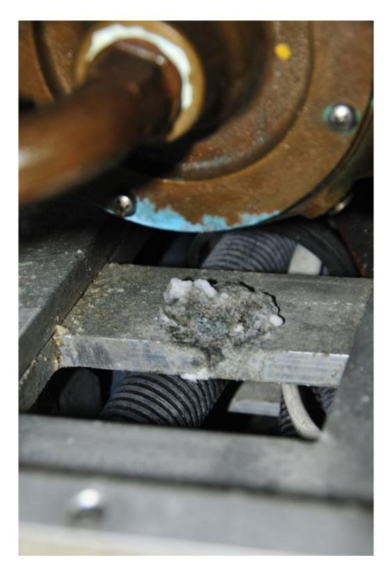
In some cases galvanic corrosion can occur even if metals are not in direct contact with each other; here water dripping from a bronze pump has corroded its aluminum support structure.
