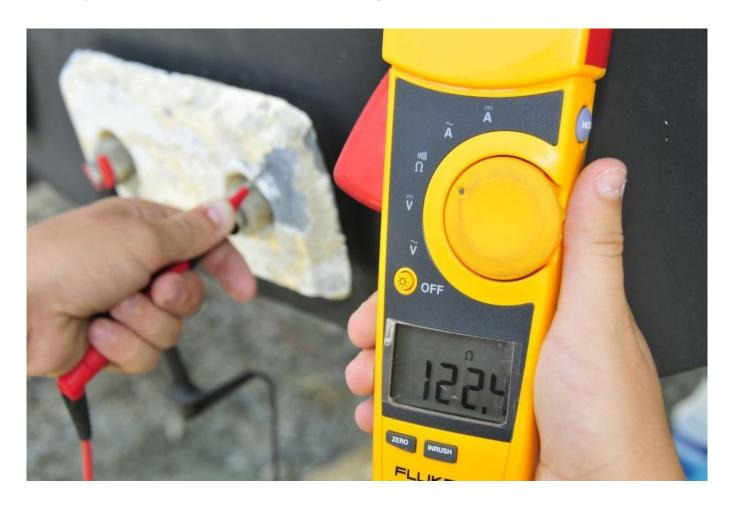
Resistance between protected underwater metals and sacrificial anodes must be kept to a minimum, no more than one ohm (this one fails to meet that standard), in order for protection to be afforded.
