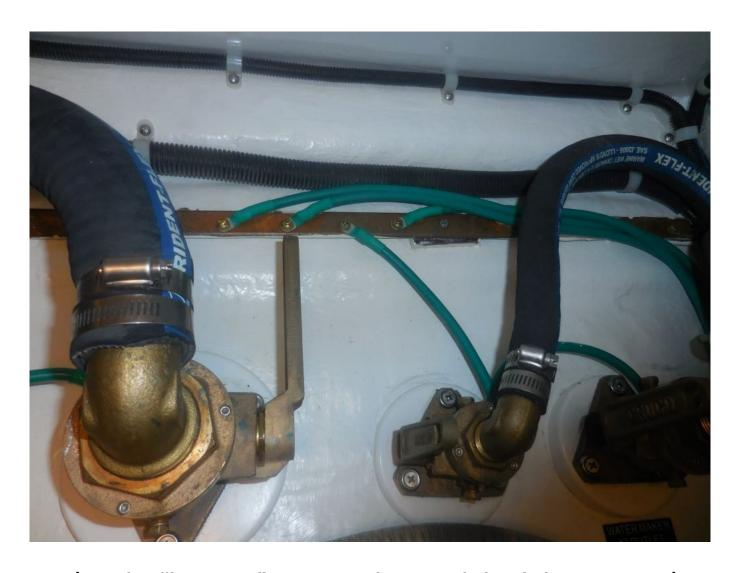
Using the "home run" system, where each bonded component is wired directly to a bonding bus, is an ideal approach that typically yields low resistance connections.
