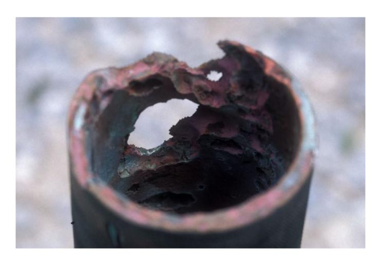
This zinc-bearing brass stern tube is suffering from dezincification, evidenced by its pinkish hue, which is a form of galvanic corrosion.
