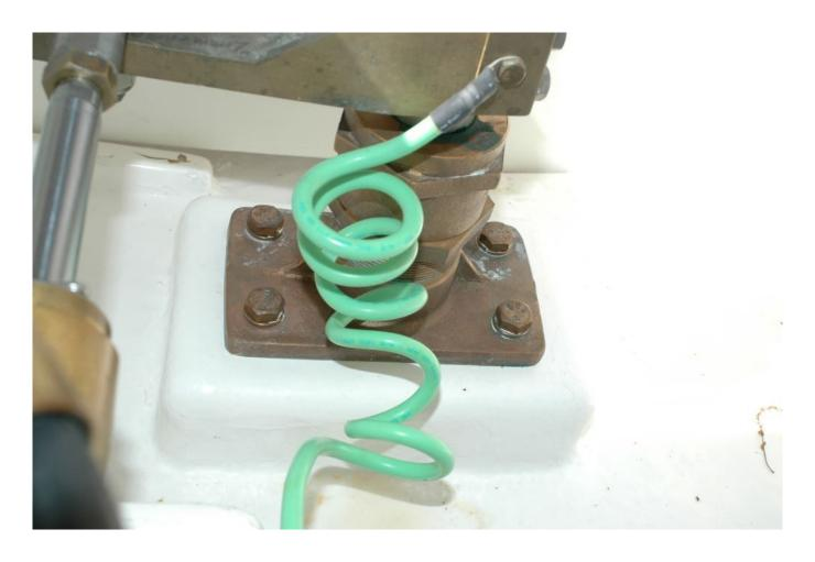
Moving components, like the rudder post shown here, require some special techniques for making long-lasting bonding connections.
