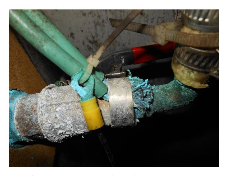
Bonding system connections live a difficult life, they are often located in bilges and exposed to water and foot traffic. Bonding connections should rely on machine screw connections, rather than on tapping screws or hose clamps.
