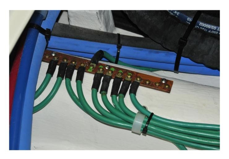
Bonding systems are an essential part of a fiberglass vessel's ability to prevent or minimize corrosion.
