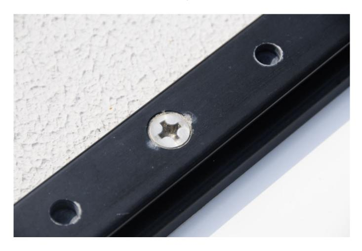
While less of an issue than some other metal combinations, aluminum can suffer from galvanic corrosion when in contact with stainless steel and water. Here, a recessed stainless steel screw traps water, setting up a galvanic cell; corrosion has already begin to set in on this new nearly boat.
