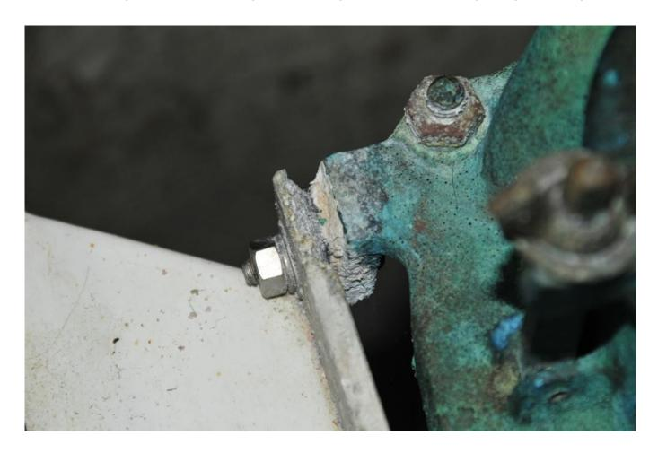
Aluminum and copper alloys like bronze are among the least compatible metals. Here a bronze raw water strainer is supported by an aluminum bracket. Airborne moisture alone would be enough to cause a problem, albeit slowly, however, every time the strainer is serviced, the two metals get doused with seawater, accelerating the corrosion process.
