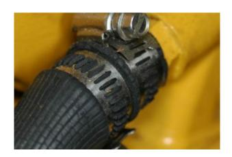
The hose used for this water heater plumbing is woefully inadequate (it is, in fact, pneumatic hose), and in spite of the short time it's been installed is already deteriorating. If this hose fails coolant will spill, and the engine will rapidly overheat.
