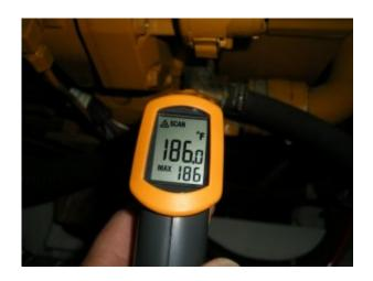
The temperature of the coolant as it leaves the engine on its way to the water heater is high, too high for safely making domestic hot water.
