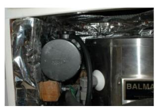
Two examples of remote expansion tanks shown above, these ensure that the highest opening in the engine's closed cooling system remains above the water heater, which prevents air from being trapped within the system.
