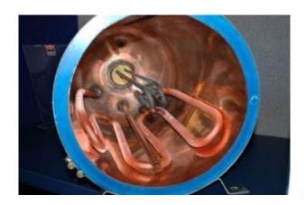
A high quality finned copper heat exchanger tube is visible inside this cut away heat exchanger, it's the long pipe making multiple S turns. The electric heating element is visible
