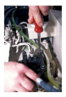
Adjustment is accomplished with a screwdriver. The locking nut is then tightened while holding the adjusting screw in place. Once that's done, the feeler gauge must be reinserted into the gap to ensure no movement
