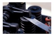
The feeler gauge being inserted into the gap between the valve stem and the rocker arm.
