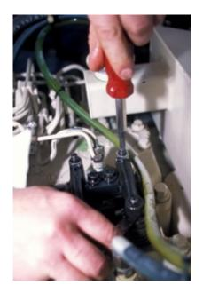
Adjustment is accomplished with a screwdriver. The locking nut is then tightened while holding the adjusting screw in place. Once that's done, the feeler gauge must be reinserted into the gap to ensure no movement has occurred during tightening.
