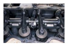
Four rockers and valve springs are seen here (two full and two partial, above). The silver shaft, on which the rockers pivot, the rocker shaft, often has to be removed in order to access all of the cylinder head bolts.
