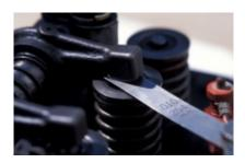
The feeler gauge being inserted into the gap between the valve stem and the rocker arm.
