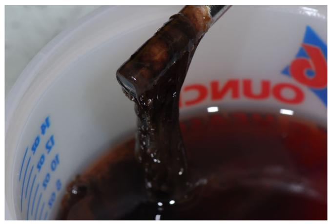
Water accumulation in diesel fuel tanks almost invariably leads to biological growth, like that shown here, and corrosion for metallic tanks, gas and diesel.
