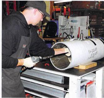
Left: The control junction modules for TRAC's stabilizer fins are complex yet reliable, thanks to the company's use of high quality materials, extensive employee training, and standardization of procedures. Right: Using specially made "extension tools," a TRAC employee installs a bow thruster flange.
