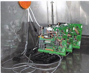
Top left: The business end of a thruster's joystick control mechanism. Because of the key role this equipment plays in vessel maneuvering, great attention to detail is paid to its design and assembly. Above left: Control cables are the "nervous system" of TRAC products and are custom-made for each project, vessel, or installation. Above right: Electronic control circuits are oven tested to ensure reliability in harsh marine environments.
