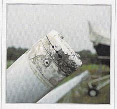
When exposed to stagnant water, aluminum can no longer maintain its corrosion-resistant oxide coating (top). Condensation dripping from a bronze water pump has caused this aluminum base to corrode (middle). Spreader tips are notorious for suffering from poultice corrosion (bottom).
