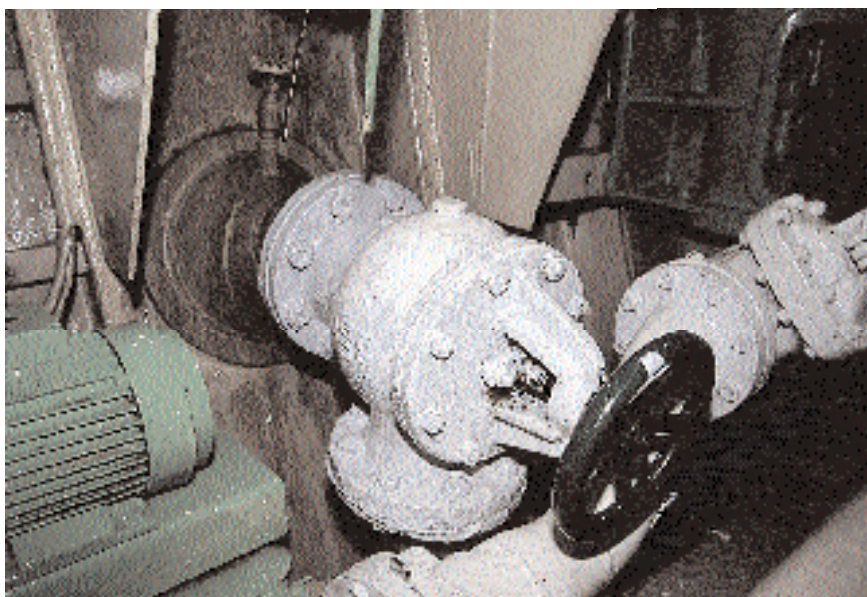
Seacocks aboard Endeavour are lubricated and exercised regularly and disassembled for inspection and service during each drydocking.
