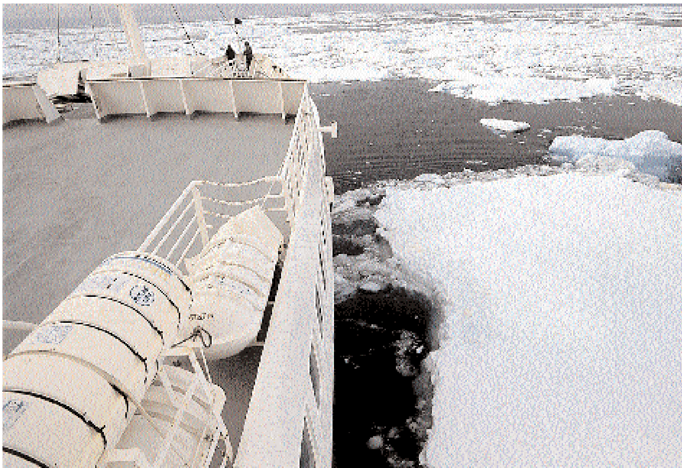
Endeavour pushes aside 100-ton ice floes with apparent ease as she traverses the Scotia Sea, between the Falkland Islands and the Antarctic peninsula. Her steel hull was designed for this type of work, albeit in Arctic, rather than Antarctic, waters.
