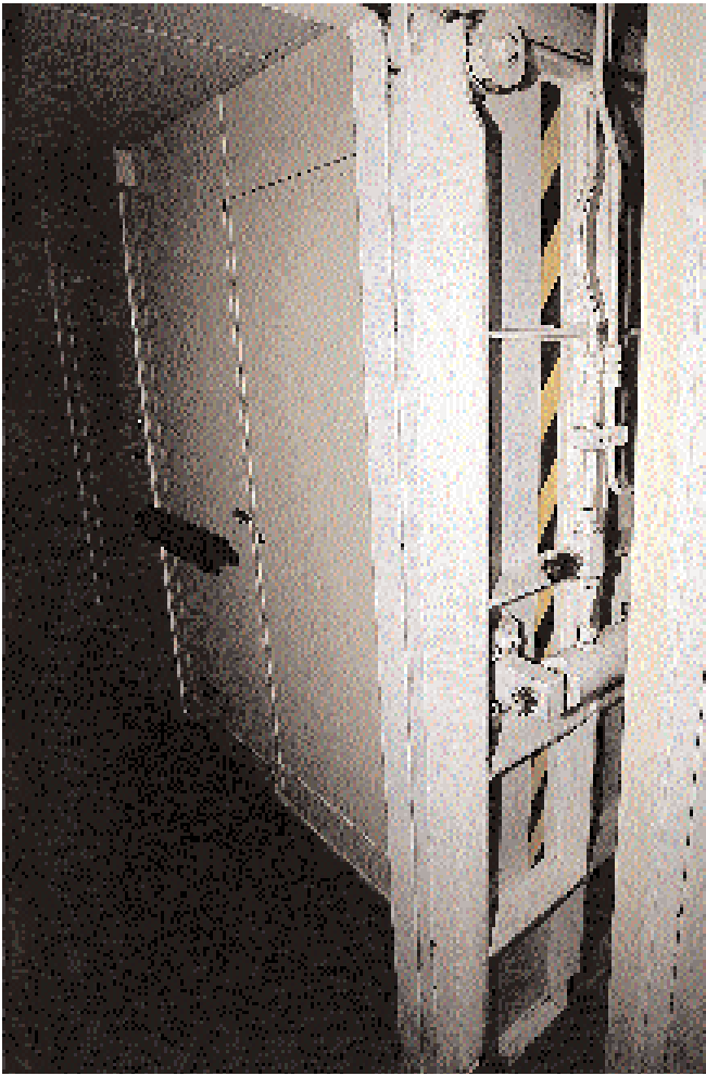
There are 10 watertight hatches located throughout the ship. These can be controlled locally or from the bridge, either hydraulically or manually.
