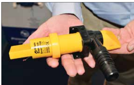
Left —A classic centrifugal bilge pump is fully submersible, tolerant of some debris, and can move a significant volume of water. Above —A low-profile, lower-volume centrifugal pump is a good option to serve as a so-called drying pump that keeps the bilge as dry as possible.
