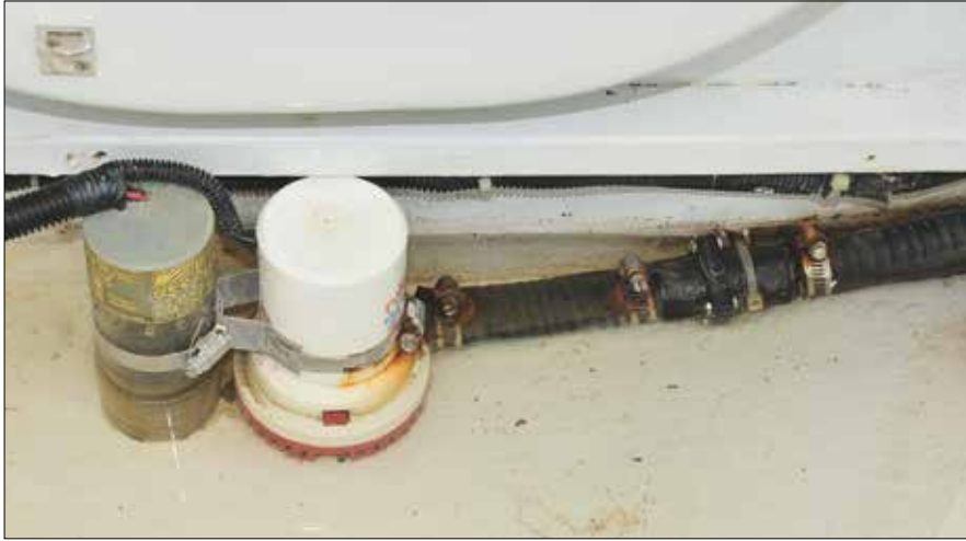
A shallow bilge can be challenging for many centrifugal pumps. Even when functioning as designed, they can leave enough water behind to cause odors and accelerate corrosion. For more effective water removal, employ a drying pump.
