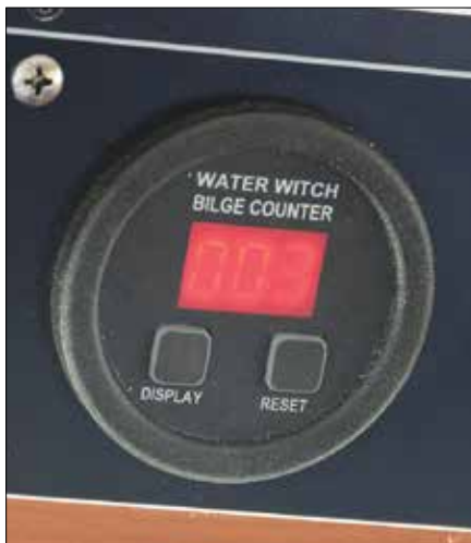
Left —All the electrical components in the bilge pump system—manual and float switches, as well as wiring—must be capable of supporting the maximum anticipated current load. This float switch overheated because it was not appropriately over-current protected and/or because it was undersized for the load the pump put on it. Right —A simple bilge counter tallies the number of times a pump cycles on. More-sophisticated models will record the duration of each run cycle as well.
