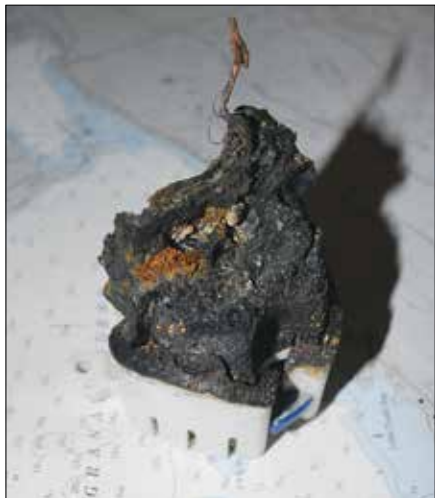
Left —All the electrical components in the bilge pump system—manual and float switches, as well as wiring—must be capable of supporting the maximum anticipated current load. This float switch overheated because it was not appropriately over-current protected and/or because it was undersized for the load the pump put on it. Right —A simple bilge counter tallies the number of times a pump cycles on. More-sophisticated models will record the duration of each run cycle as well.
