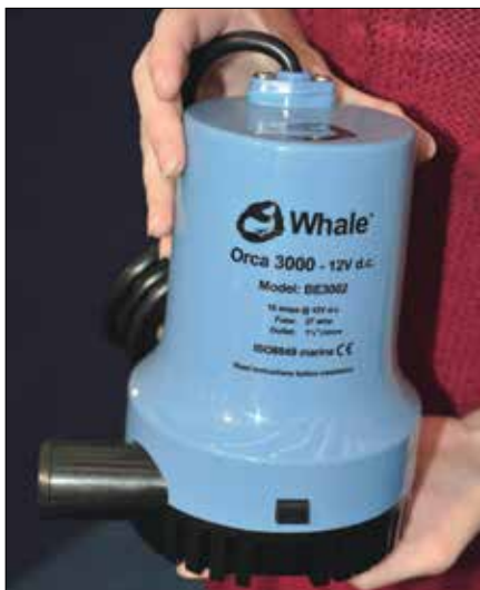
Left —A classic centrifugal bilge pump is fully submersible, tolerant of some debris, and can move a significant volume of water. Above —A low-profile, lower-volume centrifugal pump is a good option to serve as a so-called drying pump that keeps the bilge as dry as possible.
