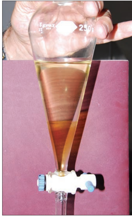
Left —VA BioDiesel's Denny Sulick displays a sample of feedstock for making biodiesel. Right —Glycerin, a by-product of biodiesel production and a versatile material in its own right, is seen here separating from the oil feedstock.
