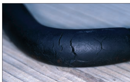
Because biodiesel degrades some rubbers and plastics, in the early '90s engine manufacturers began altering the materials in their fuel systems. Boatbuilders and tank manufacturers, as well as manufacturers of other products that come in contact with fuel, may still face a compatibility adjustment period.
