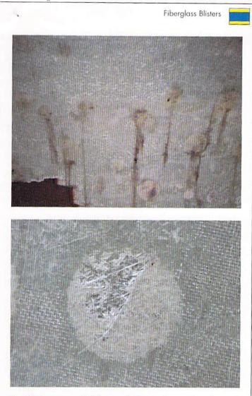
Top: Blister juice, which frequently has a vinegar-like odor and often consists of a mixture of glycol and acetic acid is seen running out of these recently exposed blisters. The acetic acid is corrosive to resin. Above: A closeup view of a blister base that's been exposed after peeling. The base of a blister may be considerably larger than its visible peak, somewhat like an iceberg, the majority of whose mass lies beneath the surface.
