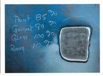
Left: A barnacle's eye view of a blister. The dome of this blister has been broken, revealing fiberglass filaments, probably chopped-strand mat (or CSM) in this case. Right: The results of a patch test tell the whole story, not a very bad one in this case. The outermost layer of fiberglass laminate is saturated; however, the layer beneath is relatively dry. The percent symbols are a misnomer, these figures are representative of a relative rather than a percent scale.
