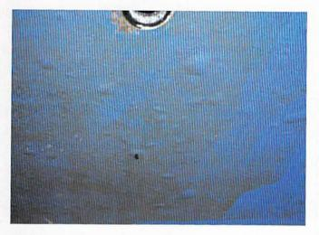
The first sign of osmosis is usually the appearance of blisters. While the quantity and size of the blisters is often an indication of the severity of the problem, a patch or lab coupon test is the only way to be certain of how deeply the laminate is affected.
