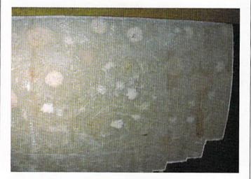
Left: This patch test reveals a previous unsuccessful blister "repair" using the spot repair, drying, and barrier coat technique. Unfortunately, the wet laminate was left behind, and the blisters themselves, the remains of which can be seen, were only ground out and filled. Right: Peeling an osmotically challenged bottom often reveals voids and delaminated areas, which must be repaired before relamination can commence. This is yet another reason to avoid the "blister repair by drying" approach.
