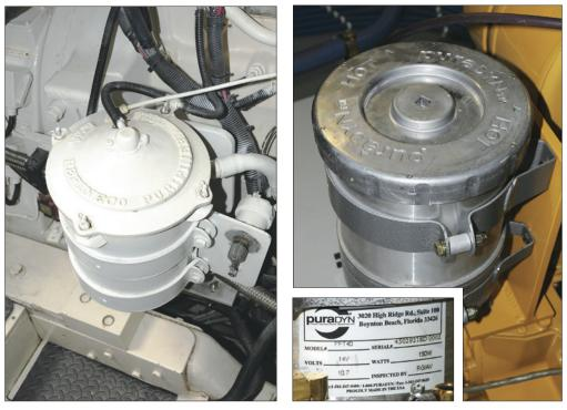
**Left**—Not factory original, this bypass filter system, like most, was added after the engine was purchased and installed in a boat. It requires little maintenance save filter replacement, and has serviced thousands of gallons of oil over the years. **Right**—This puraDYN bypass filtration system is fitted with an electrical heating element to promote evaporation of water from oil that regularly circulates at less-than-optimum operating temperature.
