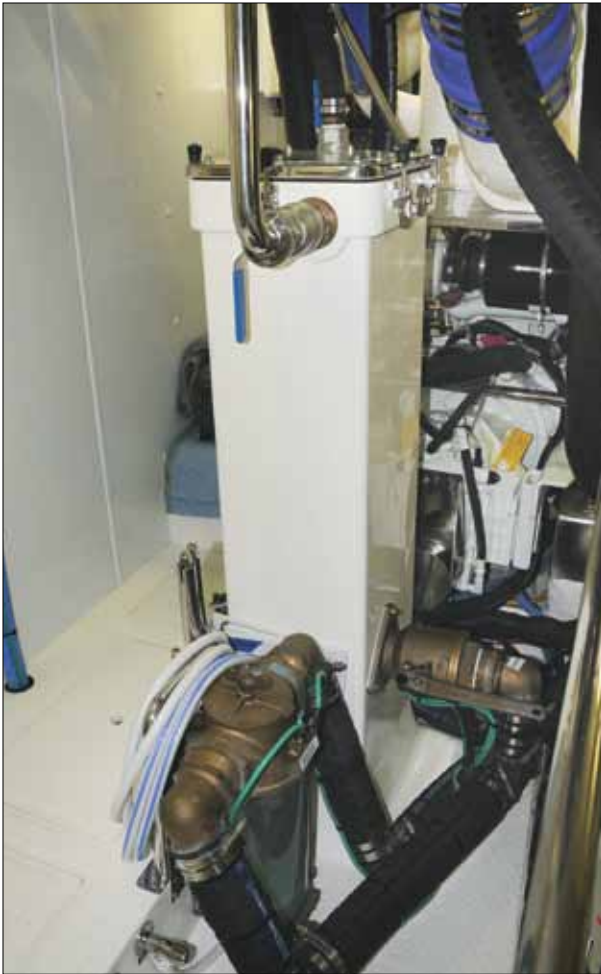
Left —The tall sea chest in the engine room is a technical complexity, but it minimizes the number of through-hull penetrations there and allows for servicing a filtering screen for the seawater intake while under way. Above —The integrated navigation system shows the vessel's track, made possible with input from the sonar system.
