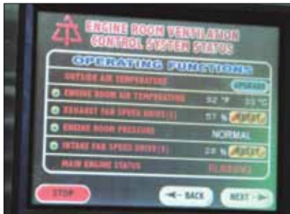
Left —Engine room ventilation was a priority, particularly because the vessel would regularly operate in the tropics. Active vents are fitted with sensors and controllers wired to a readout and control screen ( above ) at the helm.
