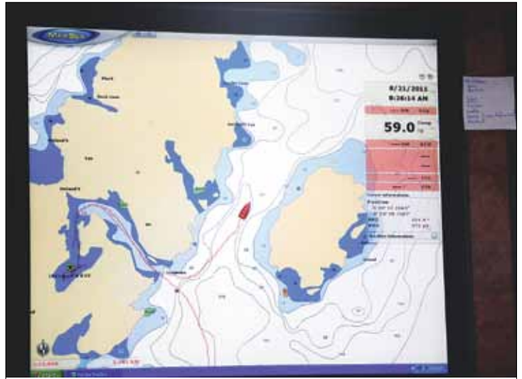
Left —The tall sea chest in the engine room is a technical complexity, but it minimizes the number of through-hull penetrations there and allows for servicing a filtering screen for the seawater intake while under way. Above —The integrated navigation system shows the vessel's track, made possible with input from the sonar system.
