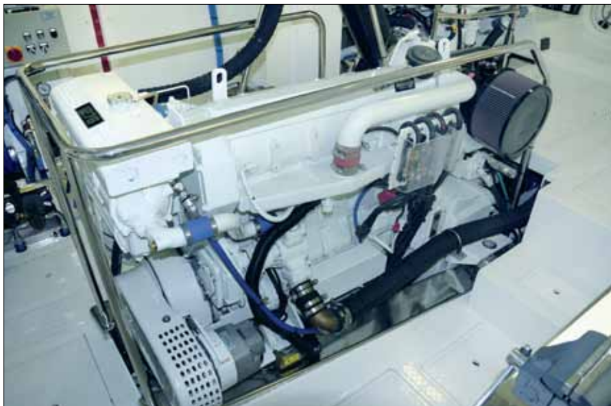
The single propulsion engine has exceptionally good access for regular inspection and maintenance. A wing, or get-home, engine provides redundancy and serves as a hydraulic pony motor.
