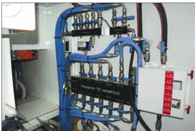
Left —For critical systems such as fuel distribution, no hose, tank, or filter should be installed until a clear plan has been established. This system is complex, but its clear labels and logical design make it easy to understand and maintain.
