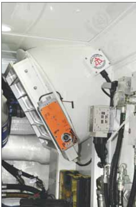
Left —Engine room ventilation was a priority, particularly because the vessel would regularly operate in the tropics. Active vents are fitted with sensors and controllers wired to a readout and control screen ( above ) at the helm.
