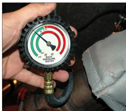
Left —Frequently, back-pressure measurements are dismissed as unimportant. Because excessive back-pressure is simply wasted horsepower, it's often incorrectly compensated for with propeller adjustments. However, exceeding manufacturer guidelines can affect emissions and void warranties. Right —To measure back-pressure, the exhaust system must be equipped with a test port in the dry section between the turbo/exhaust manifold and riser.
