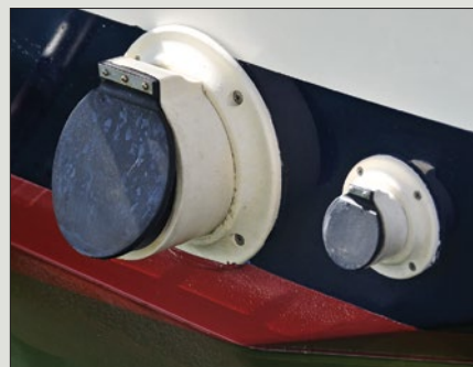
Ideally, exhaust hull penetrations should exit above the resting waterline. Flaps help minimize the likelihood of water being pushed into the exhaust from a following sea or hard backing down.
