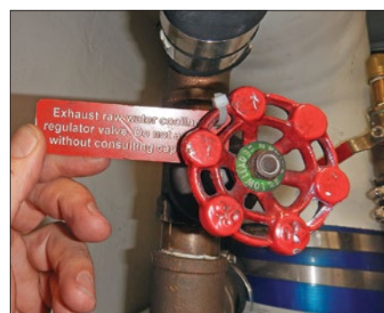
On a valve that diverts some cooling water overboard, a placard should warn against the adjustment being unknowingly changed. The handle can also be removed.
