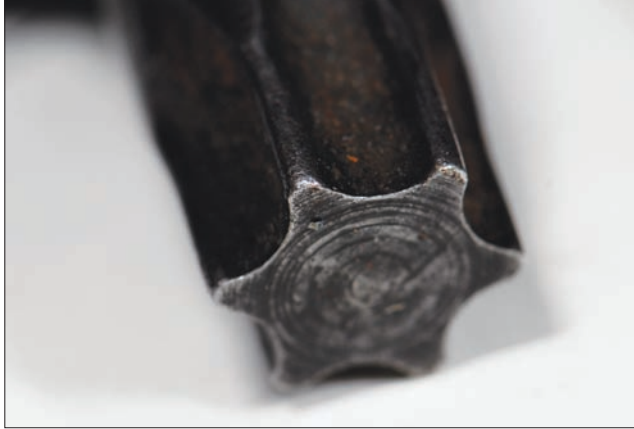
Torx, or star ( left ), and Allen, or recessed hex ( right ), drives are gaining popularity in the marine industry. These cam-out-resistant fasteners work well where there's insufficient clearance for a conventional socket drive.
