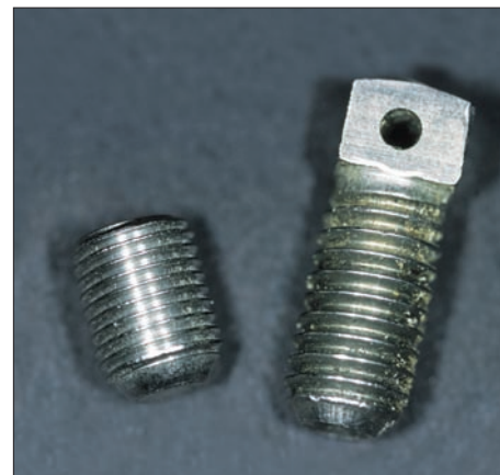
Left —An example of the wrong head. The fastener's inverted cone head acted like a simple wedge, damaging the fuel tank component. Fastener heads must be chosen as carefully as threads and dimensions. Right —Setscrews are common in marine hardware applications, and are available in a variety of types and styles. The setscrew on the right is well suited for a propeller coupling, thanks to its seizing-wire orifice. The one on the left is better for the stacked application often found on face-seal stuffing boxes.
