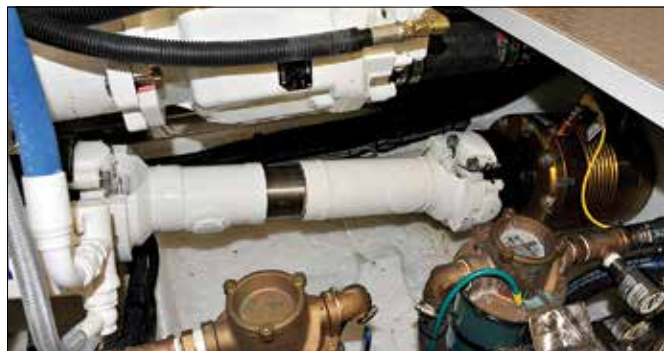
Left —Tony Fleming now field-tests new designs and equipment for the company, cruising the yachts extensively in a range of conditions and exotic locations. Above —The Seatorque shaft system on his Fleming 65 Venture was tested during a cruise to Alaska's Prince William Sound in 2013.
