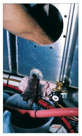
Left—Any diesel tank designed and built without a cleanout/ inspection port does a disservice to the vessel's owner or operator. Diesel tanks—even those with a polishing system—will require cleaning at some point in their lives. Below—This welding boss has been welded to an inspection port installed on an existing fuel tank, allowing a stand-alone polishing system to be retrofitted in place—without having to weld on board.
