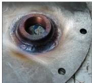
inspection port covers with a device known as a *welding boss*. The welding boss is a threaded fitting into which the pickup or return tube can be screwed. (It's easier to weld these fittings to the inspection port than directly to the fuel tank, which can be difficult and dangerous if the tank is not properly gas-freed.)
