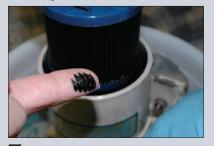
**T**heir ratings may sound "absolute," but in fact, few fuelfilter elements are precisely manufactured sieves that trap every particle over their rating size. Actually, those filter elements are designed to capture a *percentage*, albeit a high one, of all particles above a given size. Most Racor elements, for example, claim a capture rate of 90% or better.
