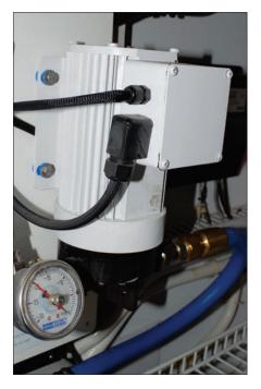
Most diaphragm pumps are quiet, can be run dry without suffering damage, and are strong self-primers.
