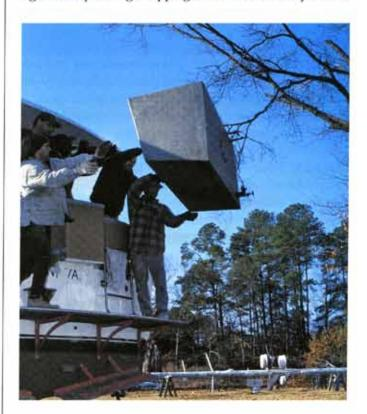
This fiberglass-encapsulated steel tank served admirably for nearly two decades. Ironically, it almost certainly would have lasted longer had it received a proper coat of epoxy paint rather than fiberglass.
