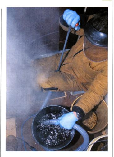
In most cases, fuel tanks cannot be thoroughly cleaned unless inspection ports afford access into each baffled chamber. This photo shows some of the debris removed from a cruiser's 30year-old fiberglass tanks after ports were added.
