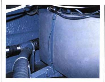
It's important to be mindful of the limitations of polyethylene fuel tanks. The most significant of these is the tanks' inability to be equipped with inspection/clean-out ports. Like most tanks, polyethylene tanks benefit from complete horizontal support. The tank pictured here is resting solely on the vessel's stringers, which is far from adequate.
