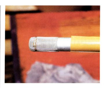
Never install a screen on a fuel pickup tube. Although this may be a well-meaning attempt at preventing clogs, it serves to do just the opposite. The preference is for debris and contamination to make its way to the primary fuel filter, where it can be dealt with easily. Clogged pickup tube screens can be cleaned only by removing the pickup tube.
