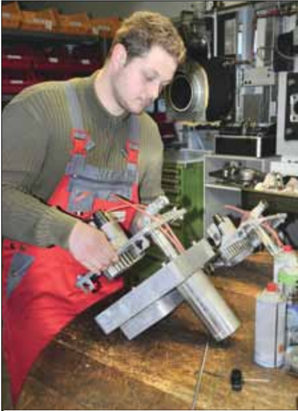
A technician at the Scheer plant in Germany assembles a burner unit. The company is known for producing some of the smallest and most efficient boilers, allowing Kabola to reduce the physical dimensions of its KB heater line—a real plus in the tight confines of a boat.
