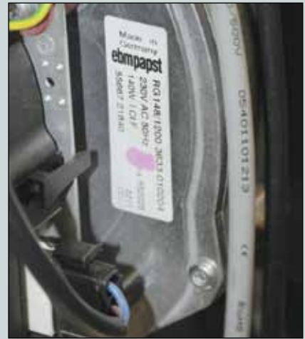
This conventional off-the-shelf blower runs on standard European 240VAC current. A small integral inverter converts shipboard 12V and 24V electricity for the furnace.
