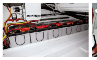
Left: While this large battery bank is easily accessible for routine inspections, it does contain a flaw; inverters should not be installed directly over batteries. Right: Batteries require ventilation for two purposes: to release hydrogen gas and to dissipate heat. This installation is conducive to neither. The "shoebox" lid will trap hydrogen gas while tightly packed batteries make heat dissipation problematic. Additionally, the tool left atop the battery presents a short circuit risk.
