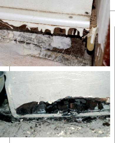
Top: The shelf on which this very large (it weighs half a ton) battery bank rests is simply inadequate. The structure must be capable of retaining the batteries in the most tumultuous of conditions. Above: Plywood, while commonly used for battery shelves and boxes, is a poor material choice unless heavily encapsulated in fiberglass resin and fabric. This box has rapidly deteriorated as a result of exposure to acid.
