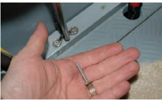
Top: While web straps can be used to secure batteries, they must be durable, robust and properly secured to the shelf or vessel. Fasteners passed directly through a strap are inappropriate for the loads that are involved. Above: Ideally, hardware used for battery security should be through-bolts rather than tapping screws. Where tapping screws are used, they must be large enough to support the load and the substrate into which they are screwed must be capable of retaining them without failure.
