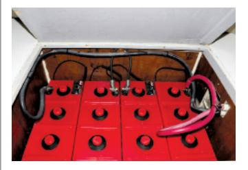
In order to allow hydrogen gas (which is lighter than air) to escape, ventilation ports must be located at the highest portion of the locker and/or box lid. This under-bunk installation fails to meet this requirement.
