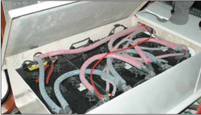
Left —Carefully install wiring for all battery banks, and mitigate the possibility of cable chafing. While the cables in this bank have been wrapped in an anti-chafe loom, its material is not ABYC compliant, because its design is discontinuous and lacks fire resistance. Right —Beyond a certain size threshold, 2V batteries wired in series make good sense because of their lighter weight, smaller size, and more manageable electrical output.
