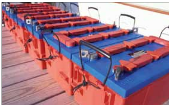
Left —When designing a bank, it's better to employ fewer larger style batteries than to a greater number of smaller case styles. This reduces the number of connections required, simplifying installation. Right —Battery specifications guide the user in building a bank of the correct amp-hour capacity as well as specifying proper over-current protection.
