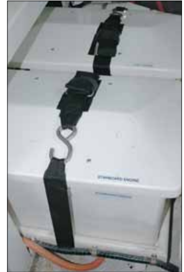
Battery boxes are ideal for securely retaining and protecting batteries and for containing spilled electrolyte. But boxes also present challenges. Chief among these is ventilation, which prevents hydrogen from being trapped within the box and allows heat to dissipate. These installations receive a failing grade because of inadequate ventilation.
