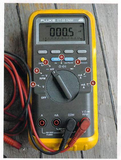
the meter pictured also measures rpm for gasoline engines.
