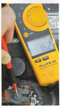
will encounter greater resistance. With navigation lights and wiring to the masthead, for instance, resistance invariably diminishes the voltage that reaches the light. (Voltage is also lost in the form of heat radiating from the wire, though this is usually an amount almost too tiny to measure.) In extreme cases, however, high resistance can and often does lead to overheated wiring, and even to fires.
