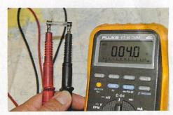
This shaft anode (far left) is making good contact with the shaft and prop, with low resistance of less than 1 ohm. The resistance between this battery lug and its adapter (middle) is higher than it should be. Resistance across a good fuse, like this one (above), should be very low, no more than a few ohms.
