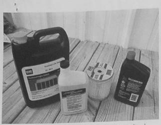
Essential engine fluids and filter, left to right: Specialized coolant that is appropriate for your engine (this is a particular issue for new diesels, which often specify proprietary nonmix coolants), hydraulic fluid for steering system, primary fuel filter element (one is never enough) and crankcase oil.
