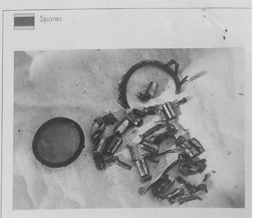
You're not likely to carry spares to resolve this failure. It's probable that the transmission these parts fell out of was destroyed because the wrong fluid was used for lubrication. It's important to carry spare parts and fluids; however, it's more important that they be of the correct type and variety.
