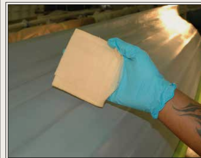
Two-part paints utilize a base and a catalyst (top left). Once mixed, the clock starts ticking, which means applicators must use their time wisely and efficiently. Paint strainers make good sense for top coats, removing debris but not the paint (top right). Tack rags are essentially sticky cloths that effectively remove dust and debris from a surface before it is painted (above).
