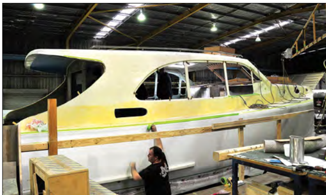
A PB 50 in construction. The drive for perfection shows in the company's emphasis on hull finish, particularly at the tumblehome in the stern quarters, because “it’s the part of the boat people look at most,” said Richards.
