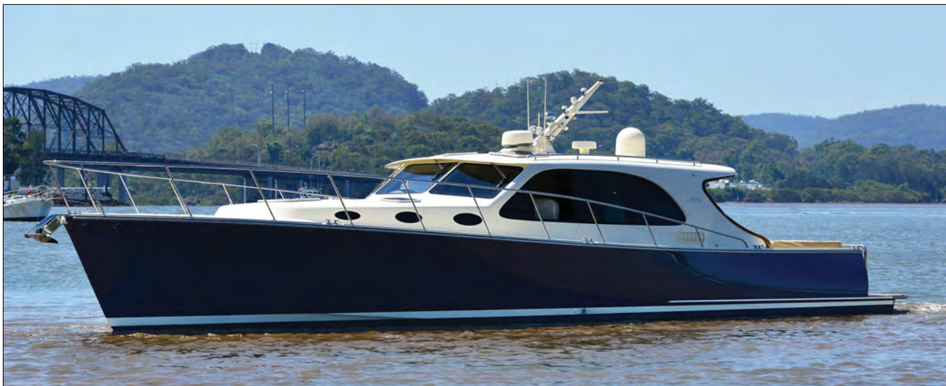
The PB 50. Richards's aesthetic philosophy for Palm Beach boats draws heavily on the "thirds rule": one-third foredeck, one-third cabin, and one-third cockpit. He's also influenced by traditional Australian designs.
