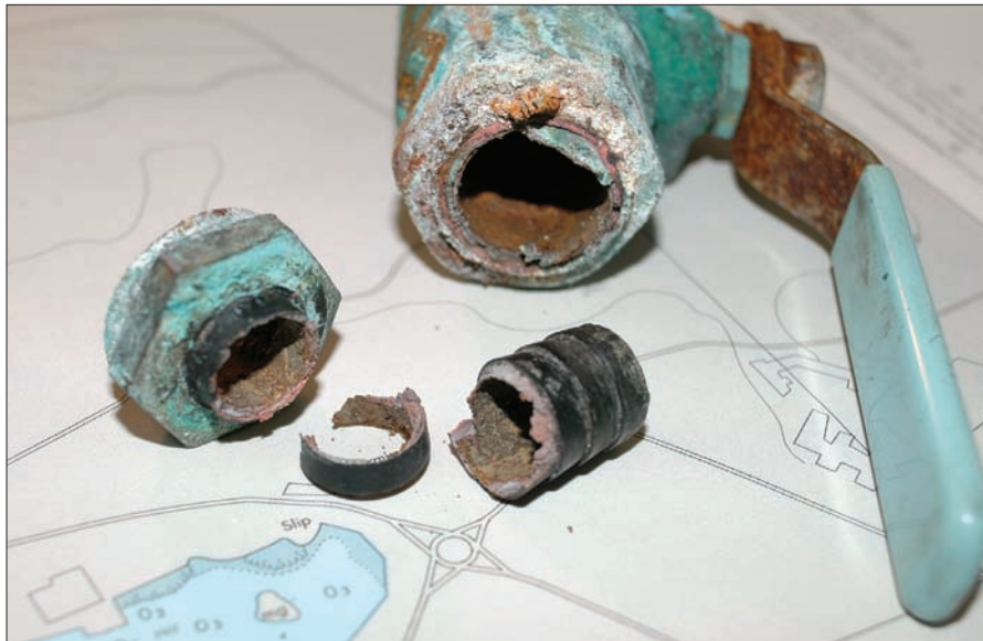
They may look similar, but brass and bronze are not interchangeable, especially in below-the-waterline applications. Owing to its high zinc content, brass often corrodes, in the process known as dezincification.
