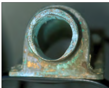
Left —While misalignment can result in the shaft making contact with the shaftlog, that doesn't necessarily cause vibration, because the misalignment is constant. However, it does create drag, leading to wear on the shaft and log. Right —Gaps and compression at bearings—like the large space between the top of this bearing and the shaft—offer clues about alignment and should not be ignored.
