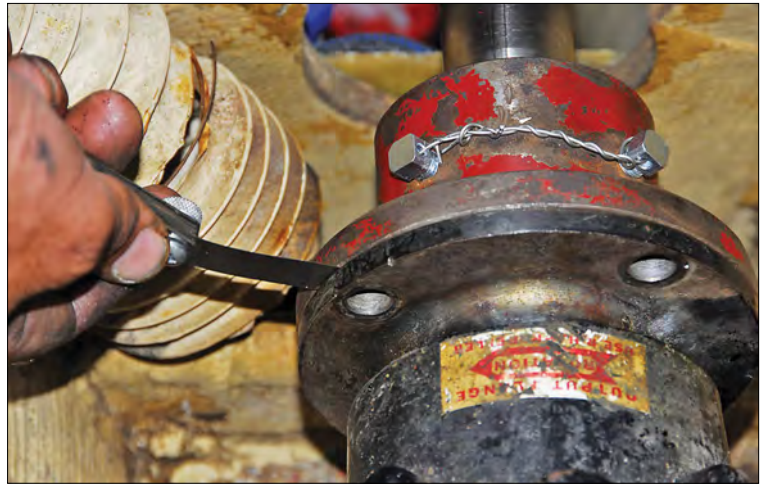
Left —An adjustable motor mount is shimmed to reduce stud extension. Boatbuilders should ensure that an initial engine installation is properly aligned without relying on excessive extension of motor mount studs, which can lead to stud failure. Instead, motor mounts should be thought of as tools for fine-tuning alignment. Above —Alignment between the engine and shaft couplings requires precise measurement, using geometry and feeler gauges, like those shown here. Ultimately, coupling faces must be made parallel and centered with each other to within a few thousandths of an inch.
