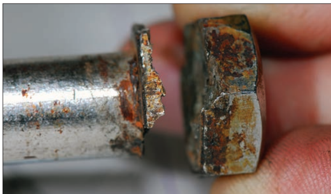
Left —This bolt's head and shank parted ways, likely from a combination of a low-quality manufacturing process and subsequent stress corrosion. Right —Crevice corrosion, occurring where the metal is simultaneously starved of oxygen and exposed to stagnant water in a bilge or stuffing box, is a common failure mode on T-bolt clamps like this one, manufactured with a metal fold that traps water.
