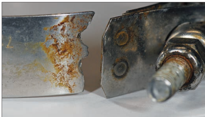
Left —This bolt's head and shank parted ways, likely from a combination of a low-quality manufacturing process and subsequent stress corrosion. Right —Crevice corrosion, occurring where the metal is simultaneously starved of oxygen and exposed to stagnant water in a bilge or stuffing box, is a common failure mode on T-bolt clamps like this one, manufactured with a metal fold that traps water.
