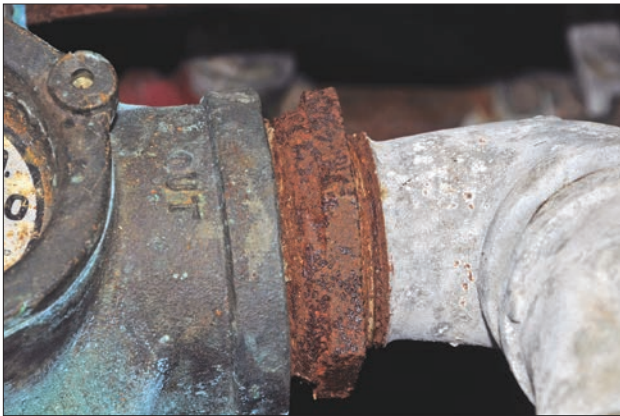
Combining mild steel, galvanized steel, and bronze in this raw-water application can lead to a variety of corrosion-induced failures.
