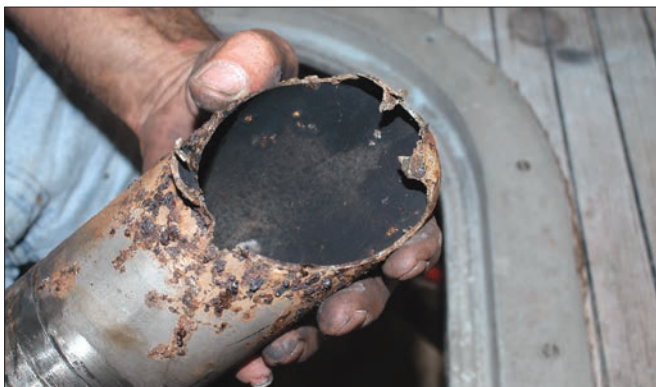
Left —Corrosion emanating from weld decay, also known as weld migration, on this stainless steel exhaust system led to complete failure. Right —Susceptibility to crevice corrosion makes stainless plumbing less than ideal for raw-water applications. In this case, the problem is amplified by the use of the incorrect high-carbon stainless alloy.
