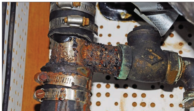
Left —Corrosion emanating from weld decay, also known as weld migration, on this stainless steel exhaust system led to complete failure. Right —Susceptibility to crevice corrosion makes stainless plumbing less than ideal for raw-water applications. In this case, the problem is amplified by the use of the incorrect high-carbon stainless alloy.
