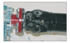
load, demanding roughly 10 times the force required by a plunging CV joint to move under the same conditions. This limits free movement of the engine and increases the undesirable transmission of vibration.
