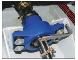
a CV joint—as the constant-velocity version is generally known—broadens the choices for engine placement and orientation. The engine can be located farther forward or farther aft, since the centerline of the engine need not parallel the propeller shaft. (Down-angle transmissions can also facilitate this type of improved installation; however, their angles are fixed, whereas a thrust bearing supports a range of installation angles.)
