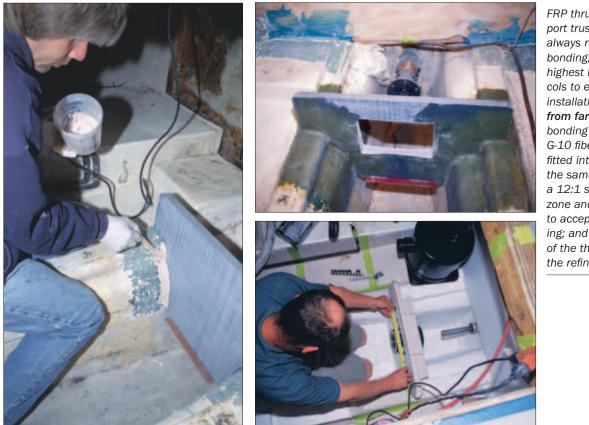
FRP thrust-bearing support trusses almost always require secondary bonding, so follow the highest industry protocols to ensure a reliable installation. Clockwise from far left—Careful bonding as a truss of G-10 fiberglass plate is fitted into an older hull; the same support with a 12:1 secondary bond zone and a cutout sized to accept the thrust bearing; and the final fitting of the thrust bearing in the refinished bilge.
