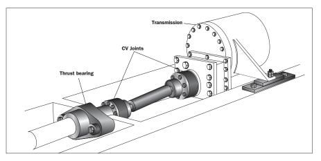
**Above**—A thrust-bearing system partially decouples the propeller from the engine by transferring propulsive thrust to structural members in the bilge, without interfering with the rotational force from the engine driving the propeller. **Right**—A cutaway of a traditional thrust bearing housed in a marine transmission. Note the tapered roller bearings and cone-shaped carrier that absorb thrust while allowing the driveshaft to spin with minimal friction.
