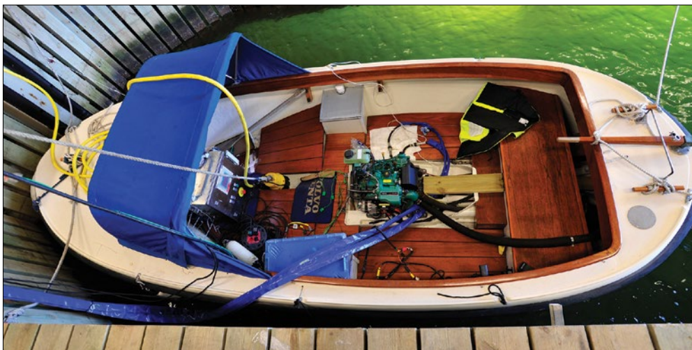
This “yo-yo” vessel is used to trial the durability of drivetrain shift mechanisms at Krossholmen, Volvo’s waterfront testing facility.
